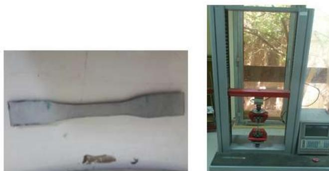
**Figure 12** Shape of Lamination Specimen Before Test **Figure 13** Tensile Test Machine
