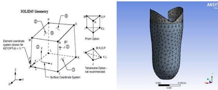
**Figure 4** Solid Element Geometry **Figure 5** The model of below knee socket with meshing
