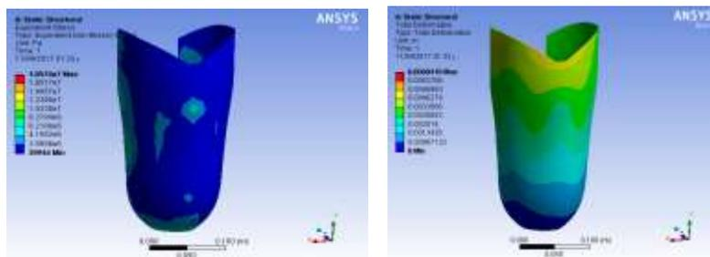
**Figure 15** Equivelant Stresses on the Socket **Figure 16** Total Deformation on the Socket
