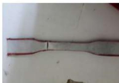
**Figure 14** Tensile Test Specimen After Test
