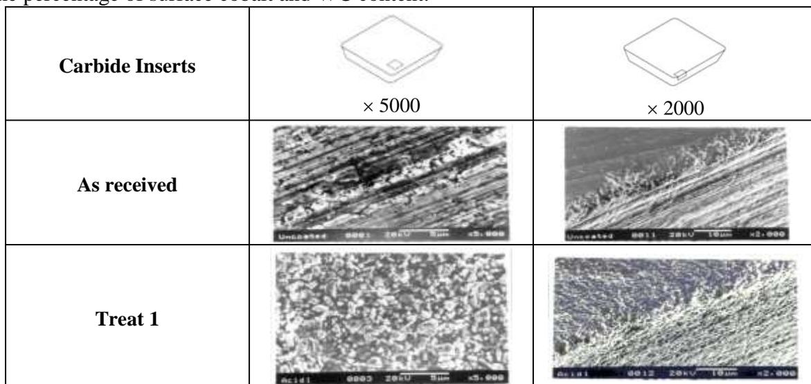
Figure 2 SEM micrographs showing the surface and cutting edge morphology of tool before and after various pretreatments.
