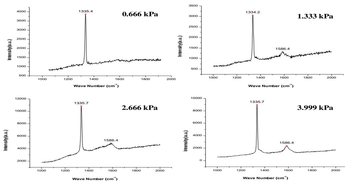
**Figure 7** Raman peaks showing the  $sp^3 / sp^2$  content with variation with deposition pressure.
