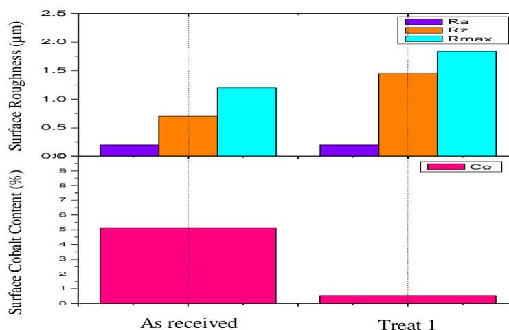
Figure 3 Surface roughness and cobalt content of WC-Co inserts surface before and after various treatments.
