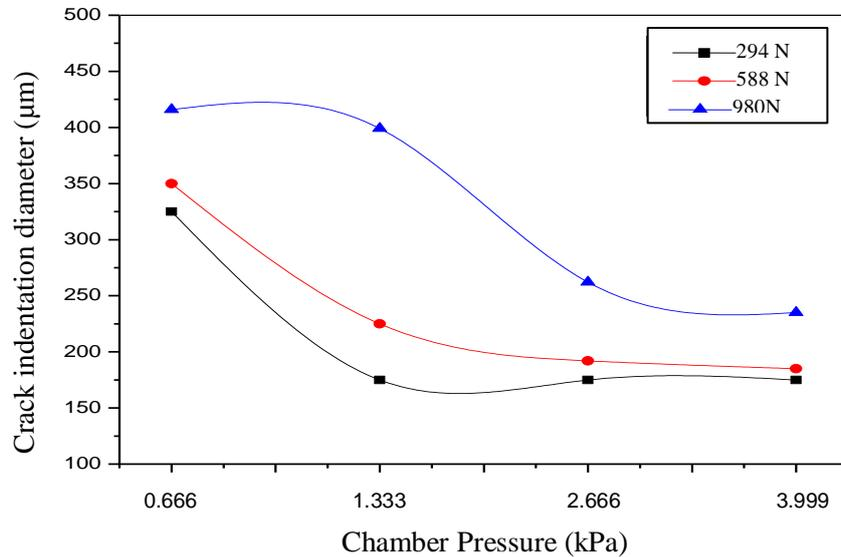
**Figure 10** Crack indentation diameter of diamond coated carbide inserts at various chamber pressures.
