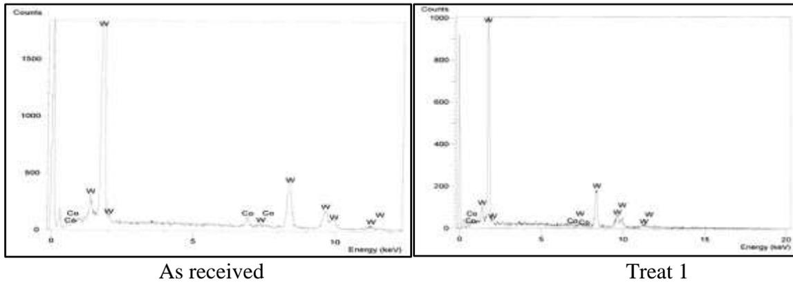
**Figure 4** EDAX spectra of the surface of as received substrate and substrate surface have undergone various treatments.
