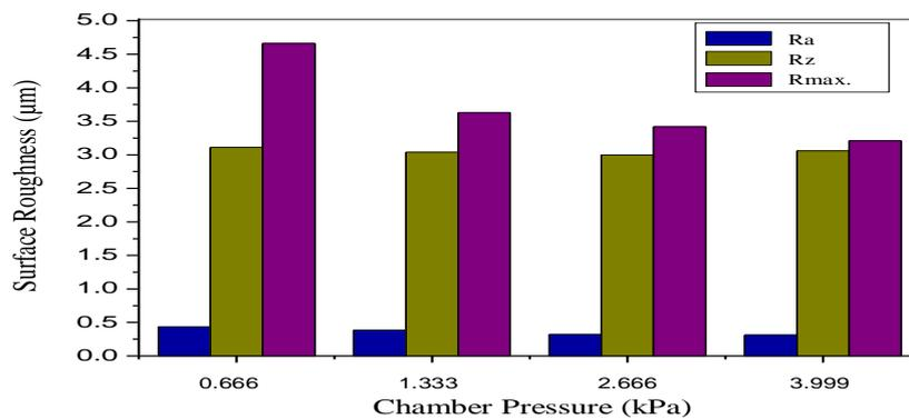
**Figure 6** Variation of the surface roughness ( $R_a$ ,  $R_z$  and  $R_{max}$ ) of the coated inserts pretreated with Treat 1 with deposition pressure.
