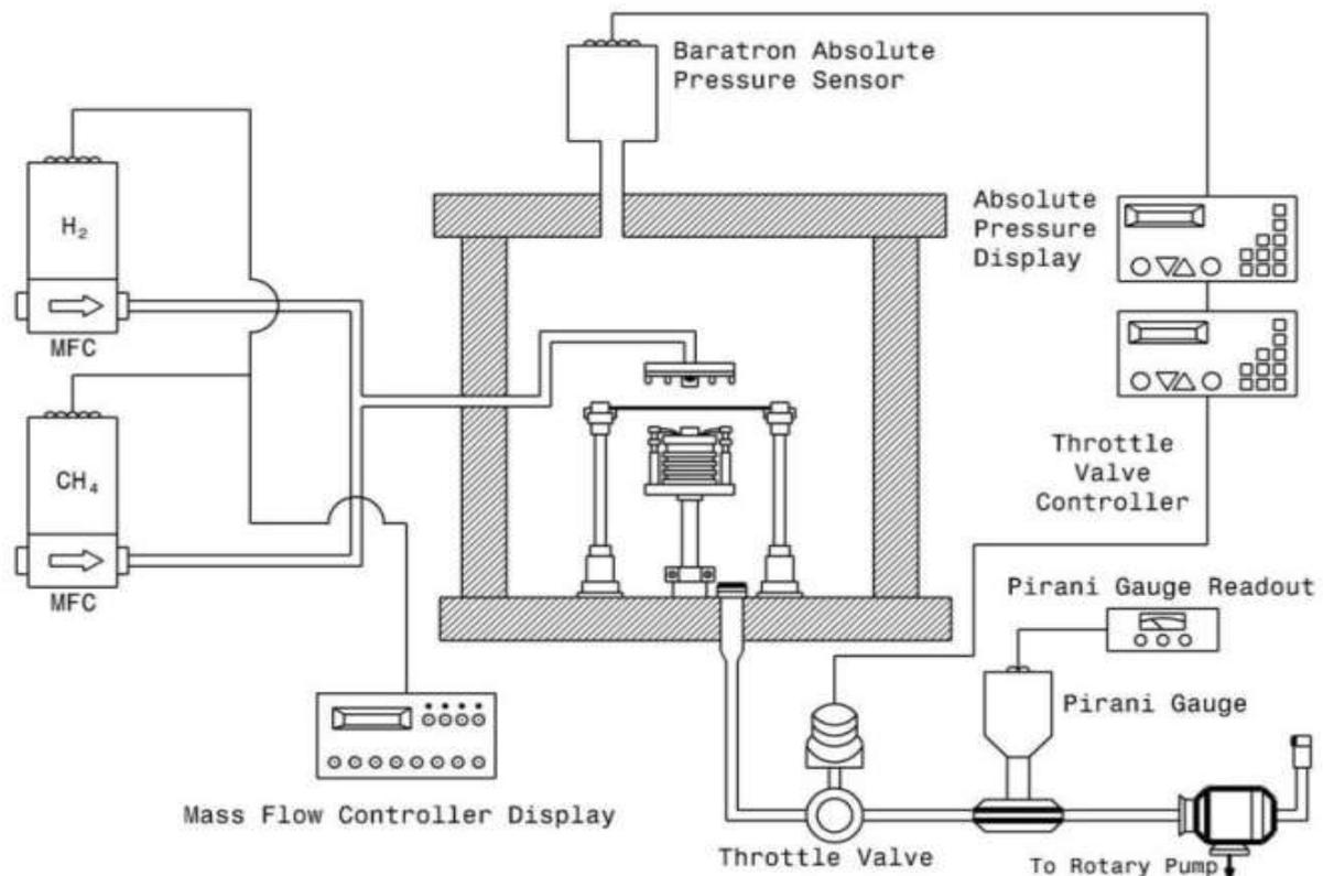
**Figure 1** Schematic view of the CVD chamber
