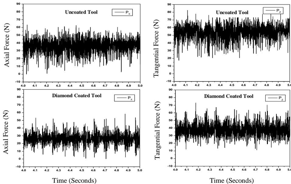
**Figure 11** Comparison of cutting forces (axial and tangential components) of uncoated and diamond coated carbide insert (Treat 1, Pressure: 2.666 kPa,  $\text{CH}_4 / \text{H}_2 = 0.5 / 100$ , Temp. =  $700^\circ\text{C}$ , Time: 8 hrs).
