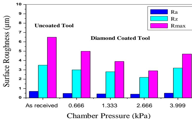
**Figure 12** Surface roughness of work-piece machined by uncoated and diamond coated inserts produced at the different deposition pressure, pretreated with Treat 1.
