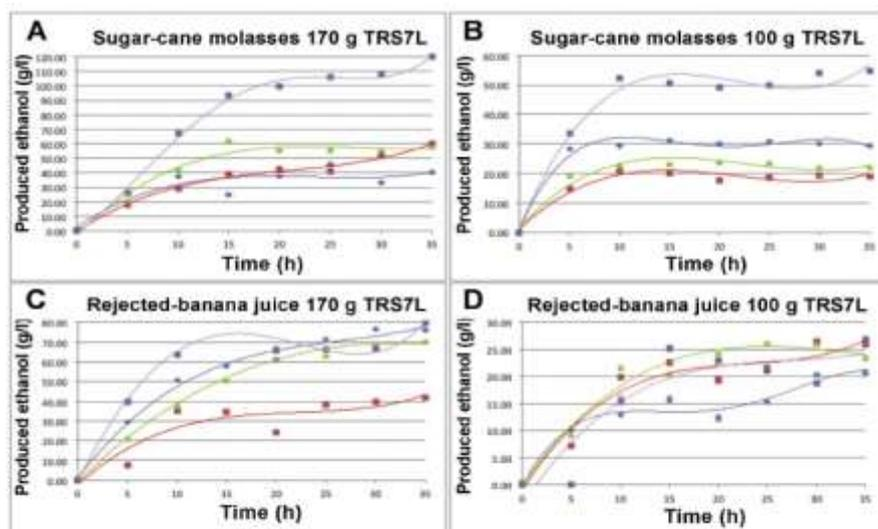
Figure 3. Kinetics of ethanol production by *S. cerevisiae* strains: CBS8066 (■), recombinant GG570-CIBI (○), recombinant GG570-CIBII (▲) and Ethanol Red® (×) under anaerobic conditions and in sugar-cane molasses with 170 (A) or 100 g/l TRS (B) or rejected-banana juice with 170 (C) or 100 g/l TRS (D)
