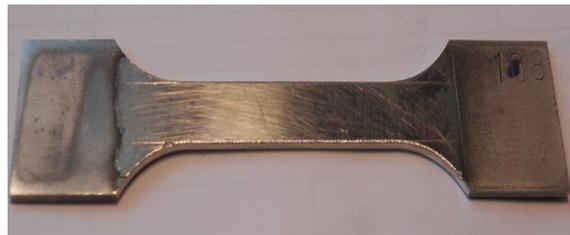
**Figure 5** Appearance of the blank after milling for static tests
