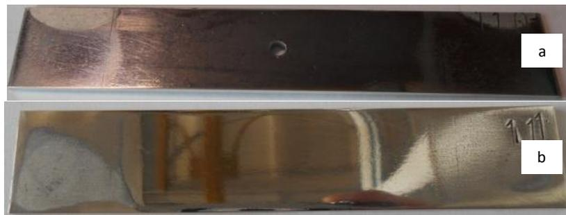
**Figure 6** Appearance of the sample after milling for fatigue tests
