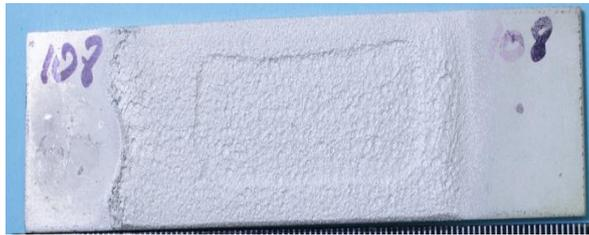
**Figure 3** Appearance of the blank with a restored area after corrosion attack
