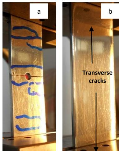
**Figure 12** Appearance of the samples after the fatigue tests
