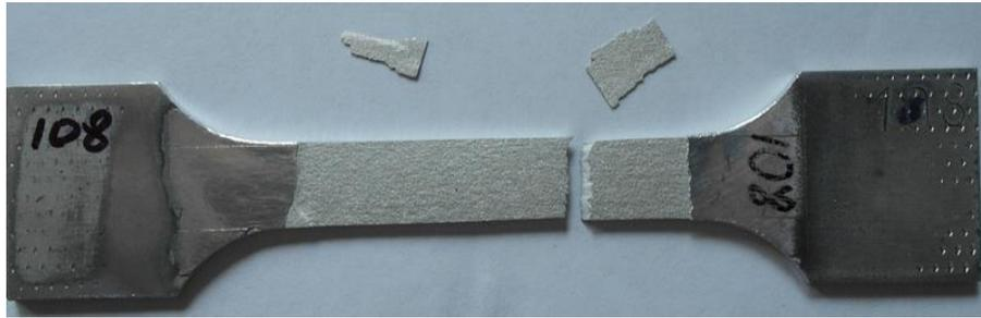
**Figure 8** Appearance of the sample after destruction in the tensile test
