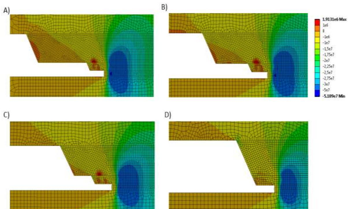
**Figure 2** Fields of stress in rock massif
