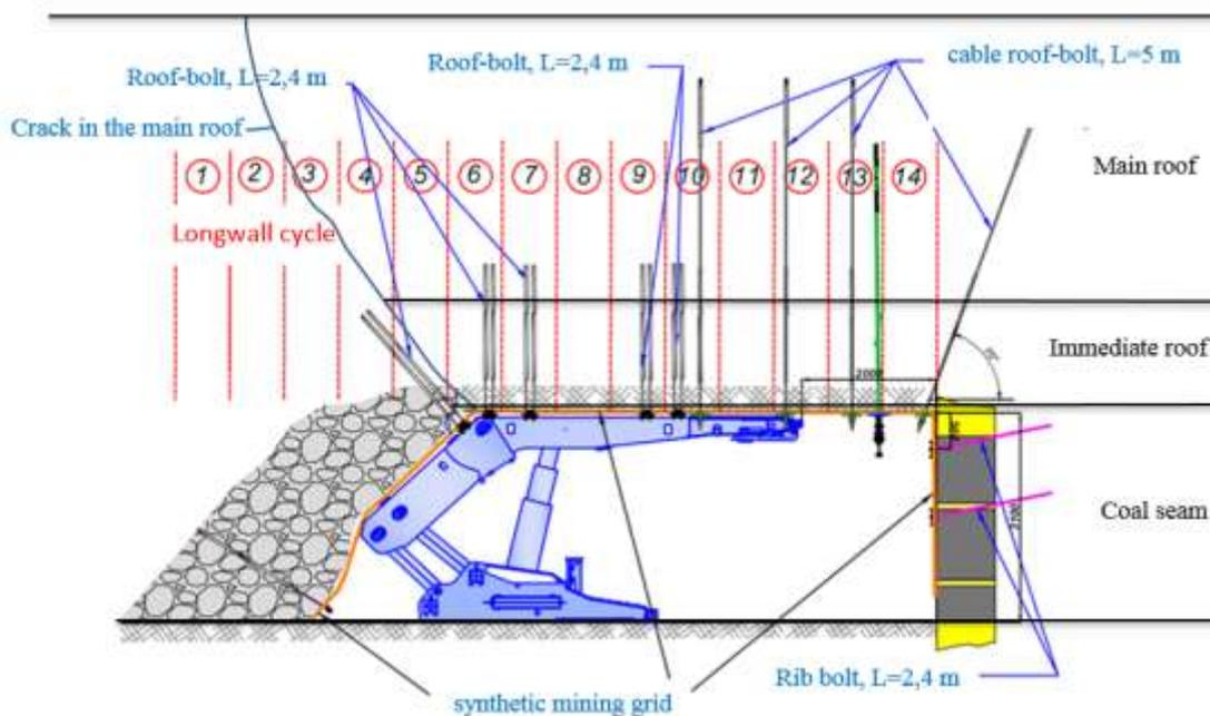
**Figure 3** Cross-section of longwall recovery room
