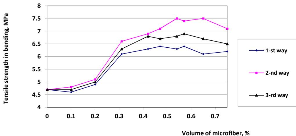
**Figure 1.** Dependence of tensile strength in bending on the volume of microfiber in different ways of microfiber introduction
