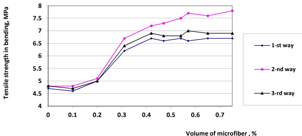
**Figure 2.** Dependence of tensile strength in bending on the volume of microfiber in different ways of microfiber introduction into rheologically active matrix
