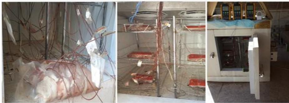
**Figure 2** Thermocouples distribution to measure meat temperature at three levels
