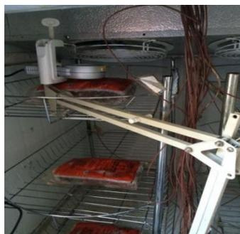
**Figure 3** Measurement of air velocity around the meat using metal vane anemometer.
