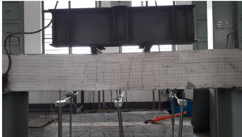
Figure 6 Test setup of a Geogrid beam
