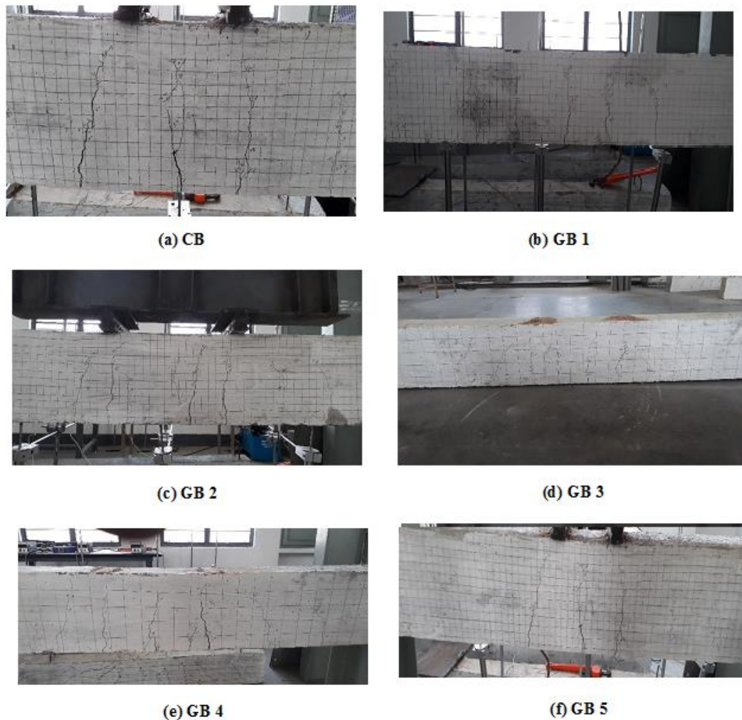
Figure 9 Crack pattern of tested beams
