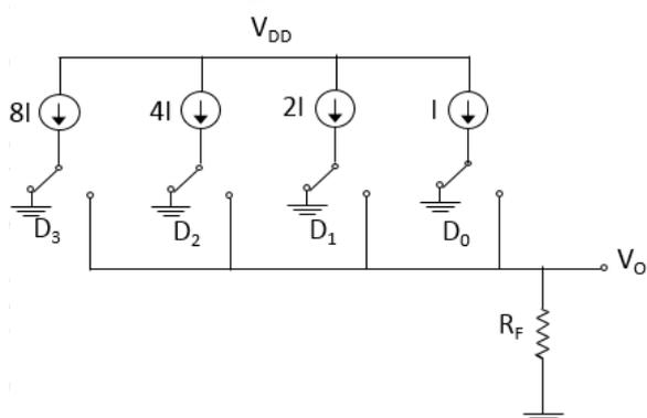
**Figure 2** 4 bit Current Steering DAC with 4 bit binary weight
