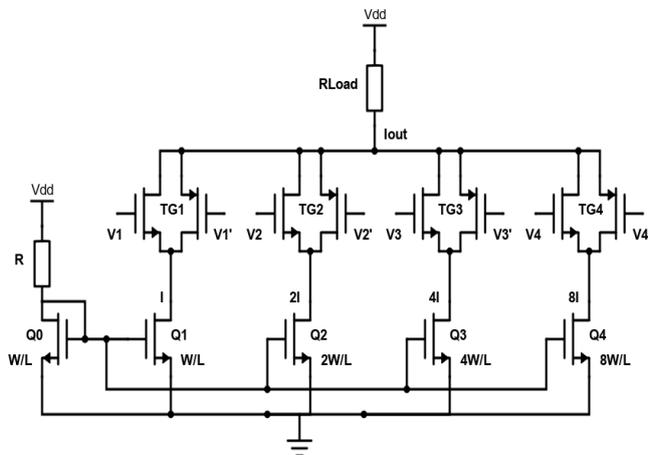
**Figure 8** Architecture of 4 bit binary weighted DAC using Transmission gate switches.
