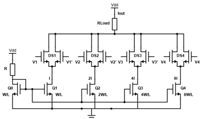
**Figure 10** Architecture of 4-bit binary weighted DAC using Differential switches [8]
