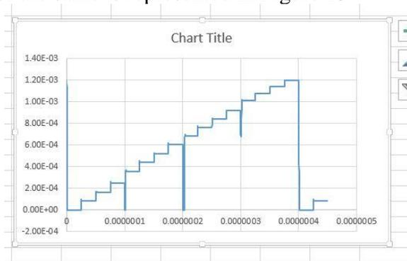
**Figure 12** Output of segmented DAC using Differential switches (LSBs are Unary and MSBs are Binary sources)
