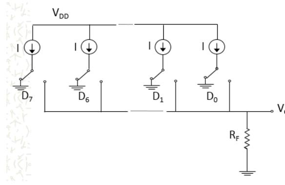
**Figure 3** 3 bit current Steering DAC with unary weight
