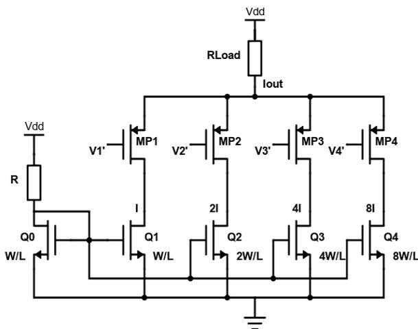
**Figure 6** Architecture of 4 bit binary weighted DAC using PMOS switches.
