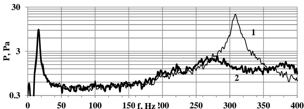
**Figure 7** Combined damping of pulsation  $P$  and force  $F_d(f)$  at 310 Hz resonance by a 335 Hz resonator in the  $P$  channel with the  $\pi/2$  phase. 1-initial signal, 2 – damping
