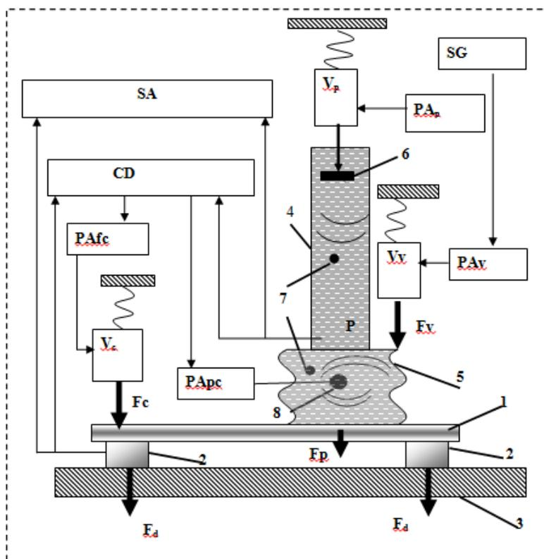
**Figure 4** Stand of two-channel AVS. CD-control device, PA-power amplifier, V-vibrator, SG-signal generator, SA-signal analyzer. Indices: c - compensation, p - pulsations, v - vibration, f – force.
