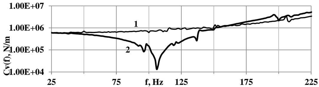
**Figure 3** Effect of water on the vibration rigidity  $C_v(f)$  of the compensator type A DN100 mm, Figure 2: 1 air (structural rigidity), 2 water
