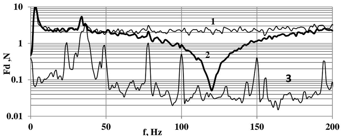
**Figure 5** Active damping the dynamic force by a resonator at a frequency of 120 Hz 1-initial signal, 2-damping, 3- interference
