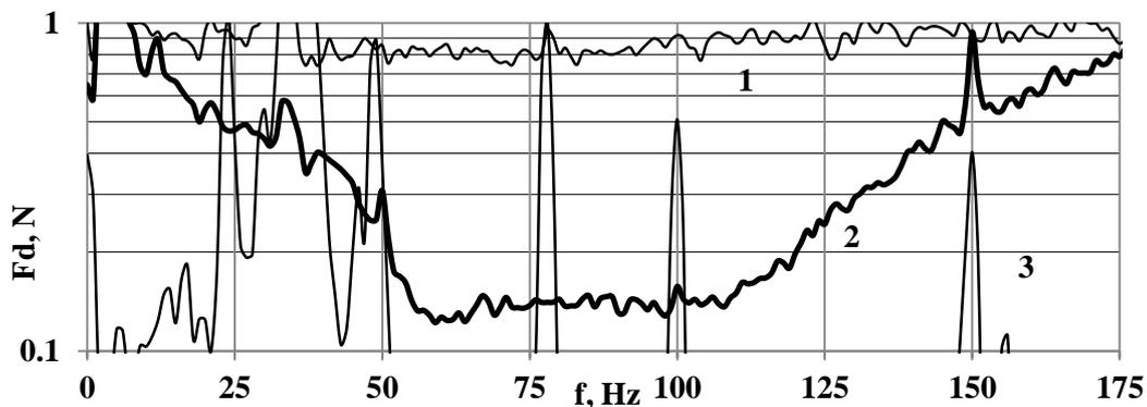
**Figure 6** Active damping the dynamic force by elliptical filters of the first order of 30-70 Hz, the second order of 50-120 Hz, and two resonators 130 Hz and 160 Hz. 1-initial signal, 2- damping, 3- interference
