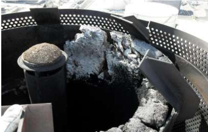
**Figure 8.1** View from above of an installed burner, with detachment of fireproof coating
