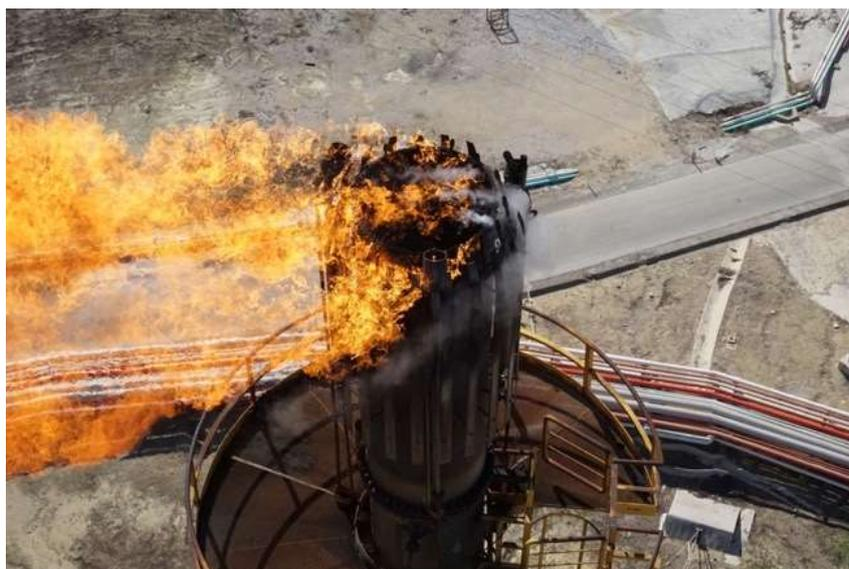
**Figure 9** Image from above the burner area (tip) of a flare stack with a defect in the steam seal using a drone
