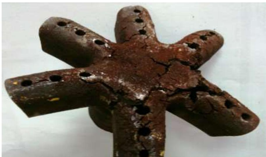
**Figure 8.3** Image of a nozzle damaged due to high temperatures
