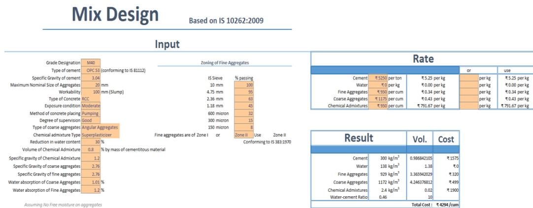
**Figure 2** Main Sheet of Spreadsheet showing Input area, Zoning of fine aggregates, Result mix and cost calculation.
