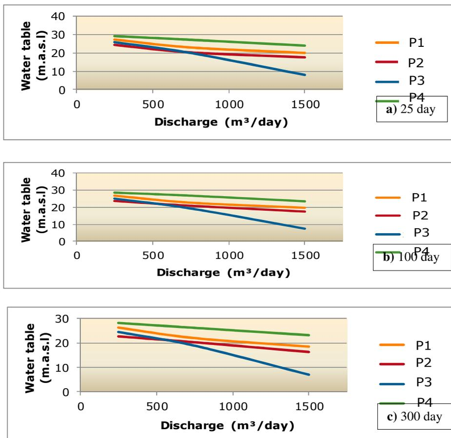
Figure (9): Discharge -Water table relationship for various running time in scenario -3
