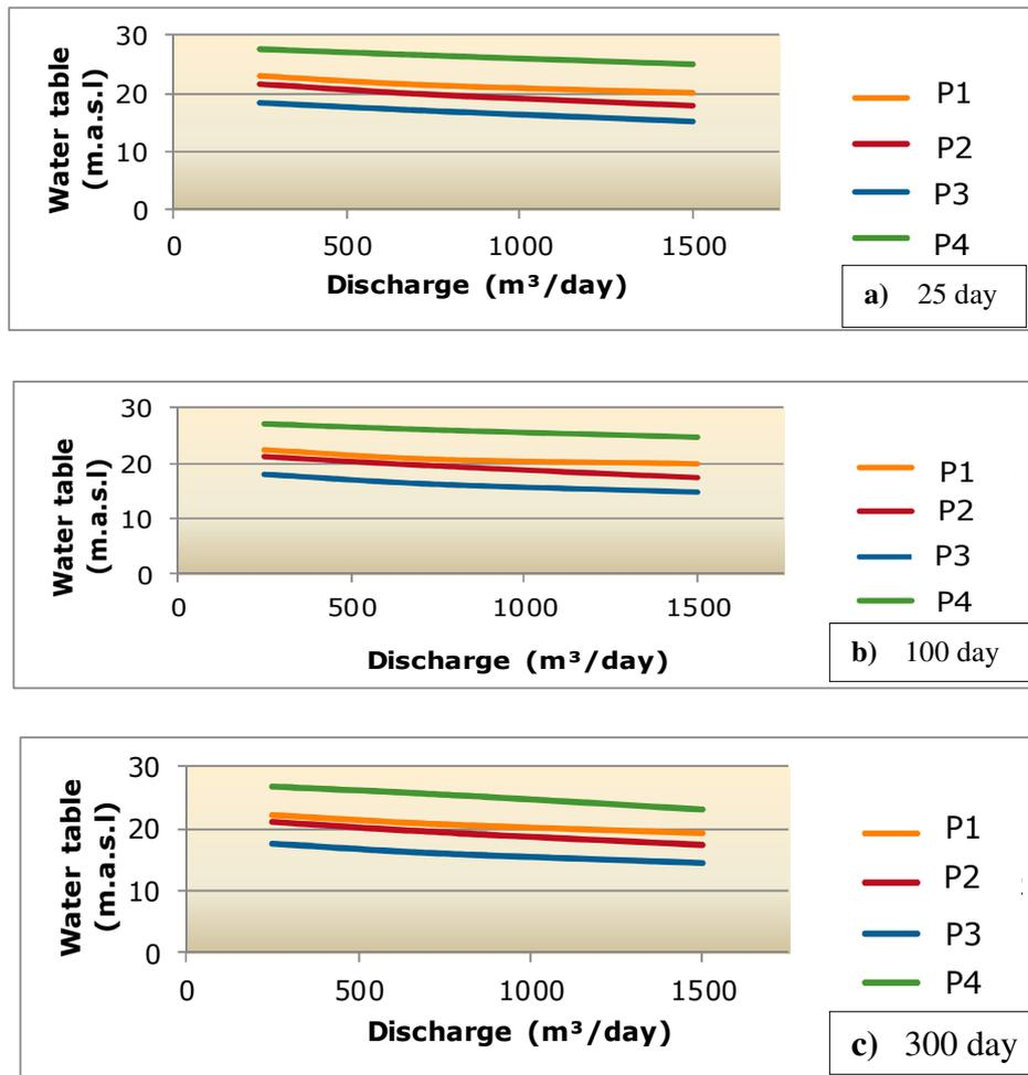
Figure (7): Discharge -Water table relationship for various running time in scenario -1
