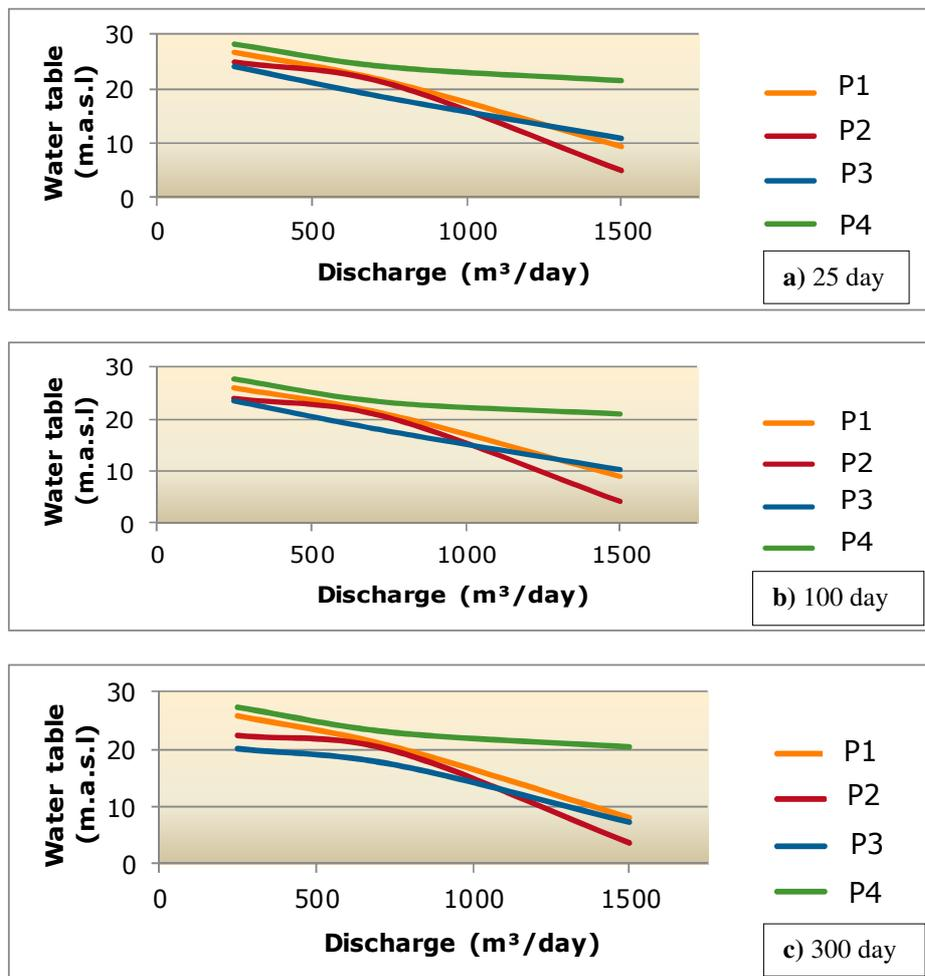
**Figure (10):** Discharge -Water table relationship for various running time in scenario -4
