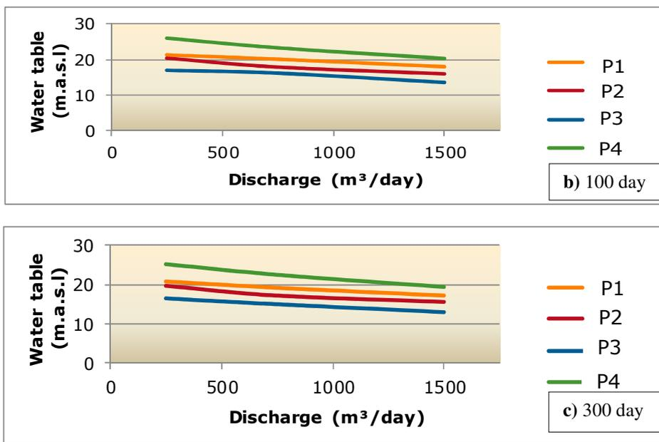
Figure (8): Discharge -Water table relationship for various running time in scenario -2
