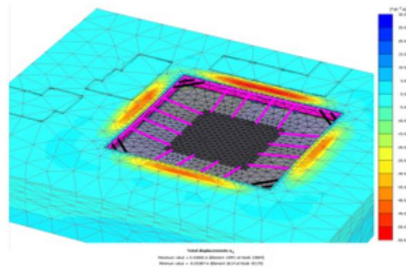
Figure 5. Final stage. Vertical displacement isopoles
