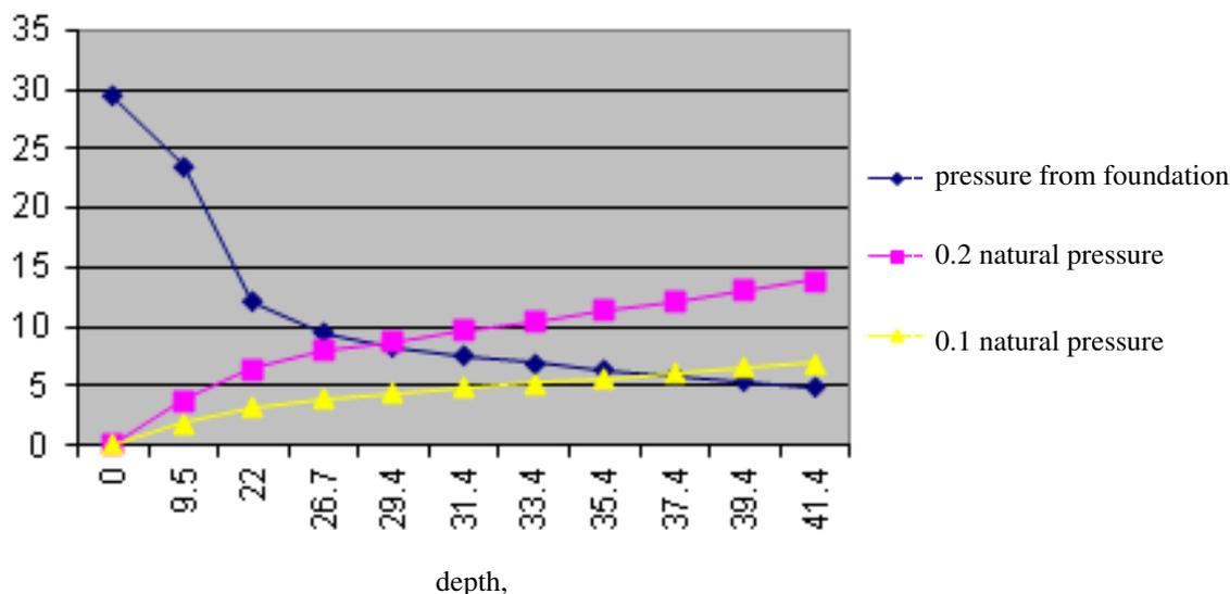
Figure 7. Results of calculations of the foundation settlement
