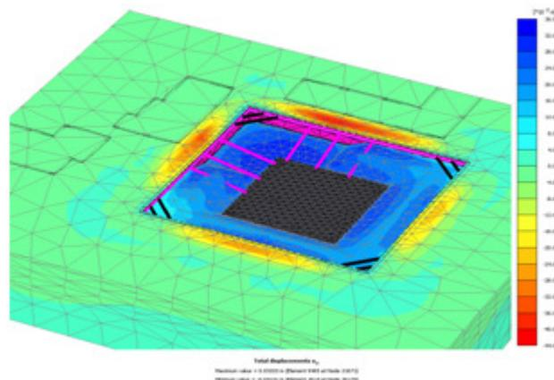
**Figure 4.** Vertical displacement isopoles. The main stage of the foundation pit construction. Development of sectional grip berms, consecutive incorporation of struts
