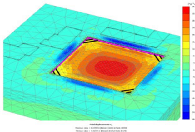
**Figure 3.** The preparatory stage of the foundation pit construction. Building soil berms. Vertical displacement isopoles
