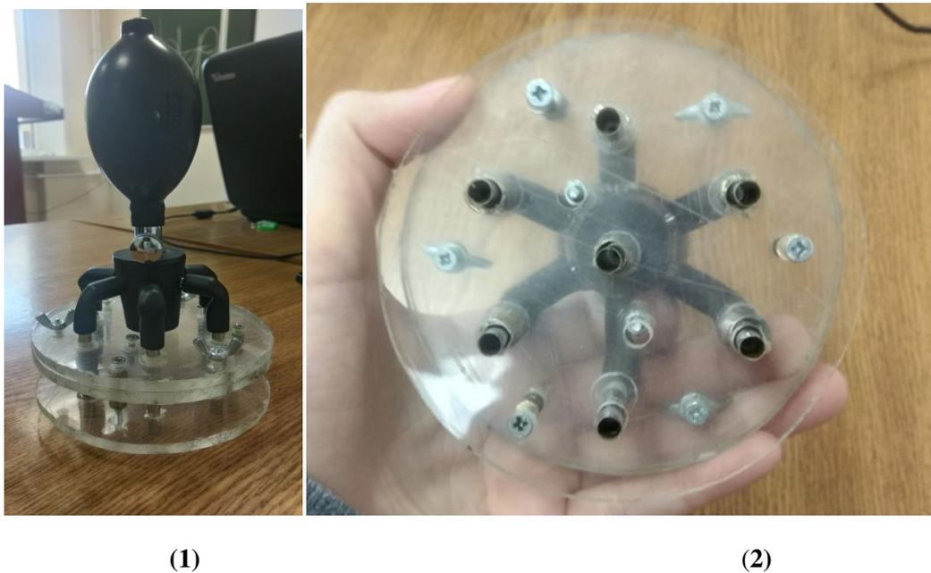
**Figure 2** The experimental model of the microbiological punch (1 – side view, 2 – bottom view)
