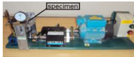
Figure 3 The Shape of Fatigue Specimen Figure 4 Fatigue Test Device.
