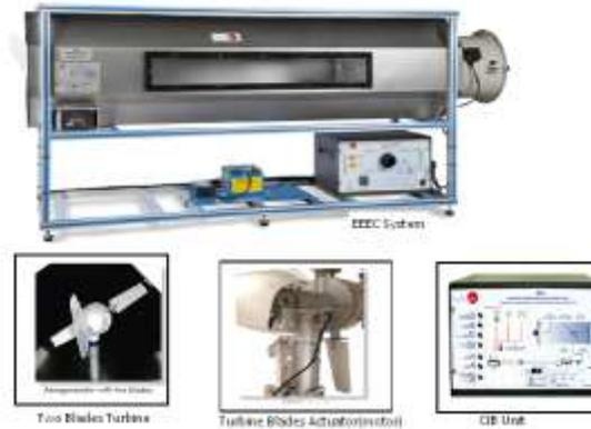
**Figure 1** Shows System Components
