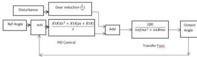
**Figure 10** System with PID Controller
