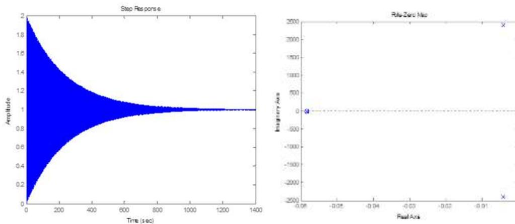
**Figure 8** Simulation Response due to  $K_p=6000$ ,  $K_i=350$  **Figure 9** Pole Locations due to  $K_p=6000$ ,  $K_i=350$
