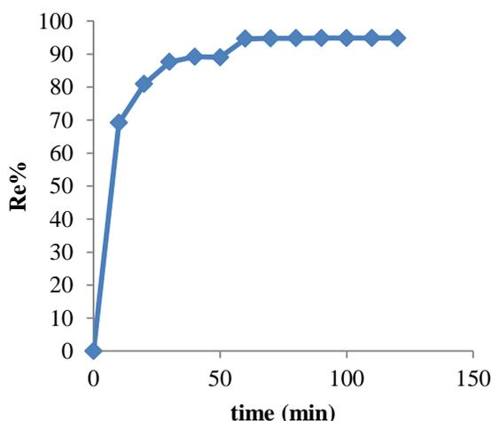
Figure 4: Effect of time on Cu (II) uptake.
