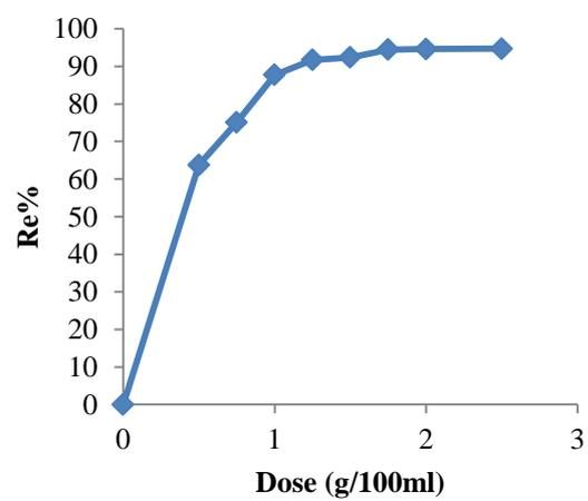
Figure 3: Effect of sorbent dose on Cu (II) uptake.
