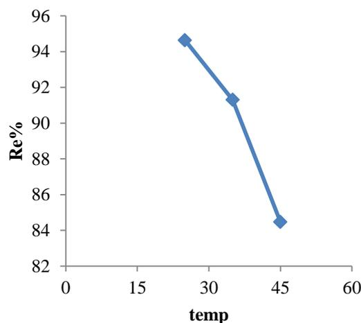
Figure 5: Effect of temperature on of Cu (II) uptake.
