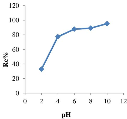
Figure 2: Effect of pH on of Cu (II) uptake.
