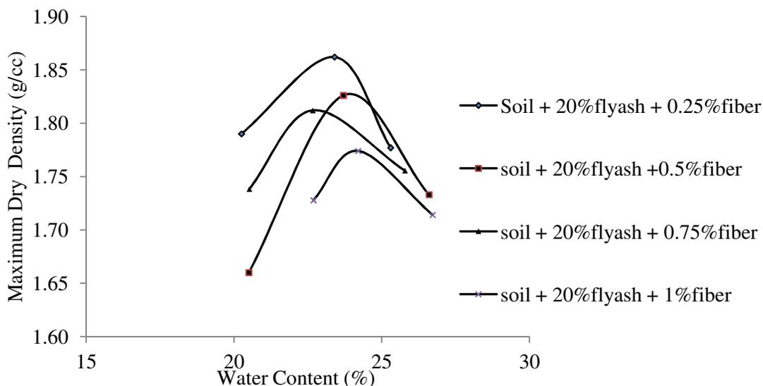
**Figure 6** Compaction Curve of Black Cotton Soil With 20% Flyash and Different Percentage of Fiber
