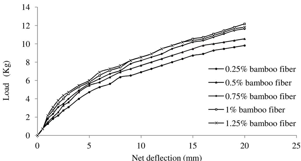
**Figure 2** Load deflection curve of black cotton soil mixed with optimum percentage of fly ash and different percentage of Bamboo Fiber
