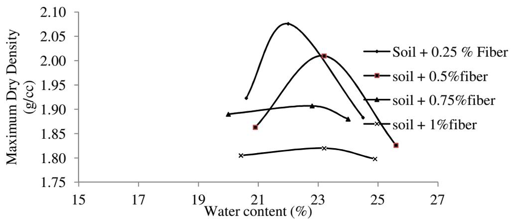
**Figure 4** Compaction Curve of Black Cotton Soil with Different Percentage of Fiber
