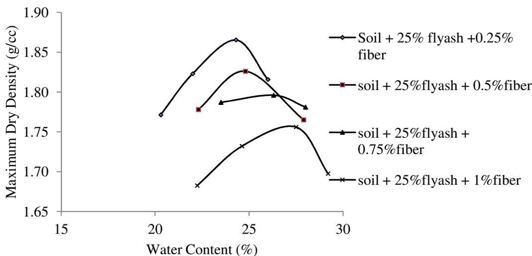
**Figure 7** Compaction Curve of Black Cotton Soil With 25% Flyash and Different Percentage of Fiber
