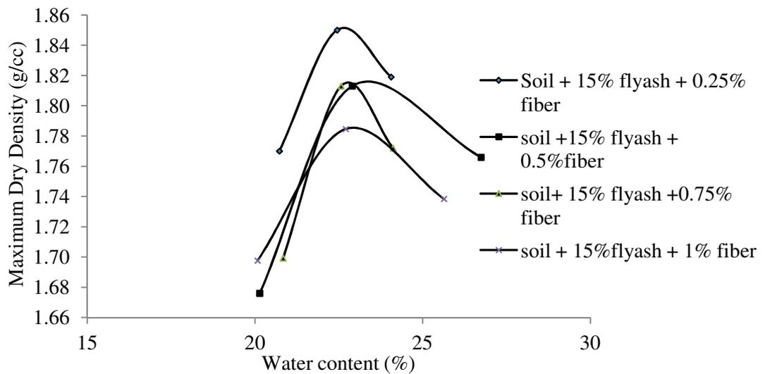
**Figure 5** Compaction Curve of Black Cotton Soil with 15% Flyash and Different Percentage of Fiber
