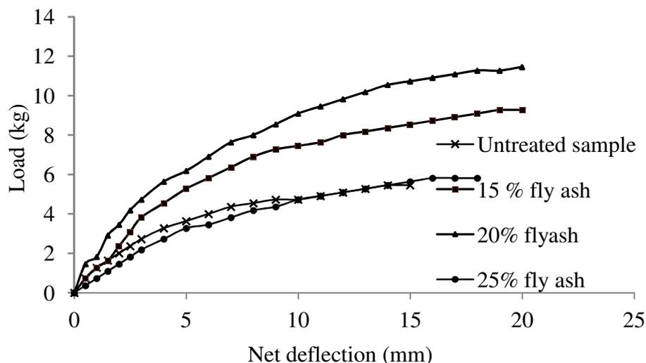
**Figure 1** Load Deflection Curve of Black Cotton Soil Mixed With Different Percentage of Fly Ash
