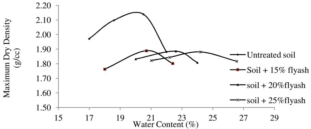
**Figure 3** Compaction Curve of Black Cotton Soil with Different Percentage of Flyash
