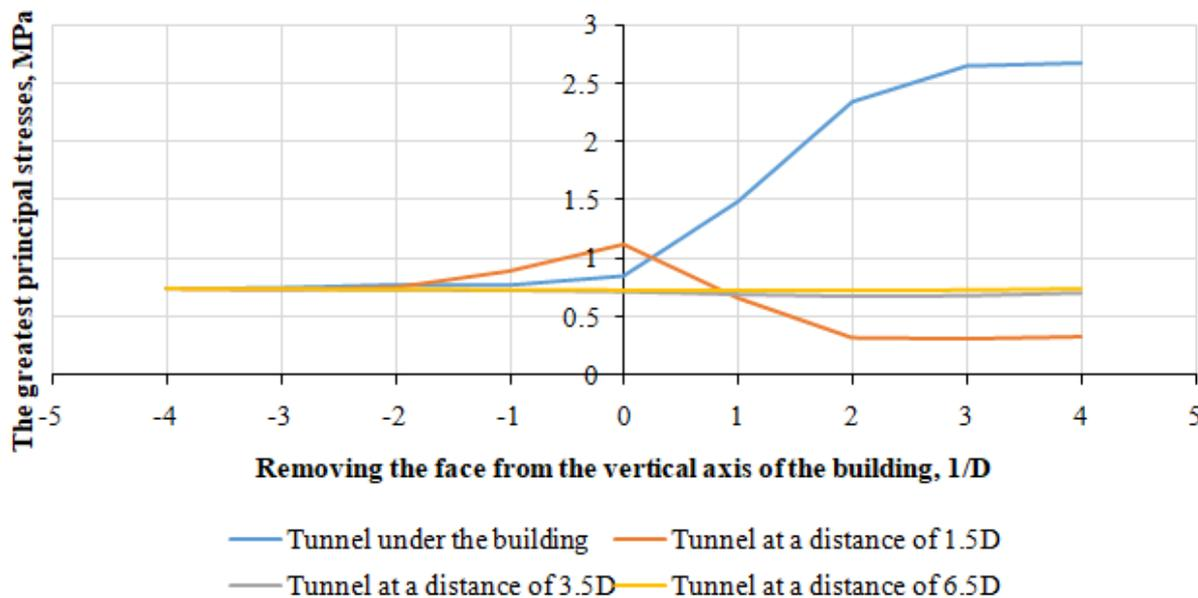
**Figure 2.** Development curves of the largest main stresses in the lower part of the building wall as the tunnel face moves
