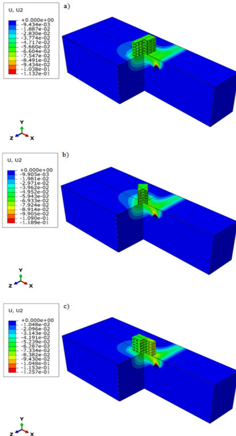
**Figure 1.** Isochromes of vertical subsidence of earth surface with different orientation of the tunnel towards the building, m. a) along the building; b) at an angle of 45°; c) along the building
