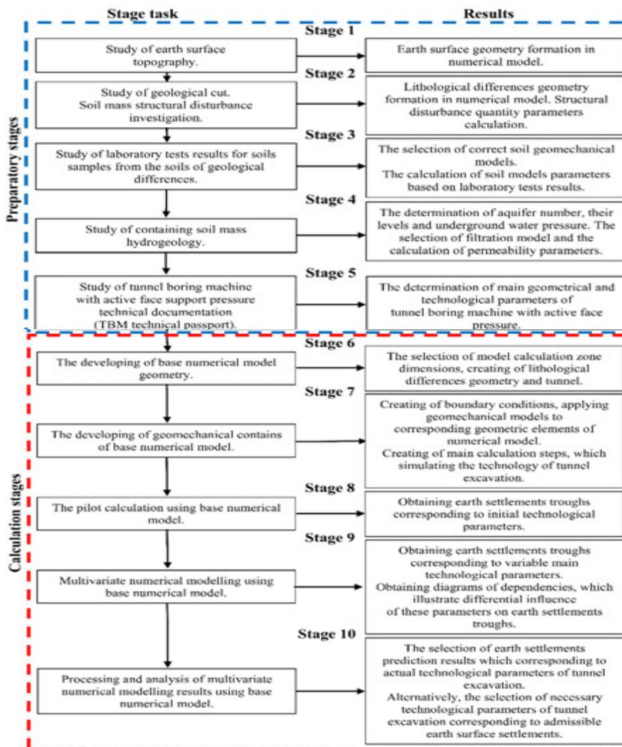
Figure 3. A flowchart of the method of predicting earth surface subsidence
