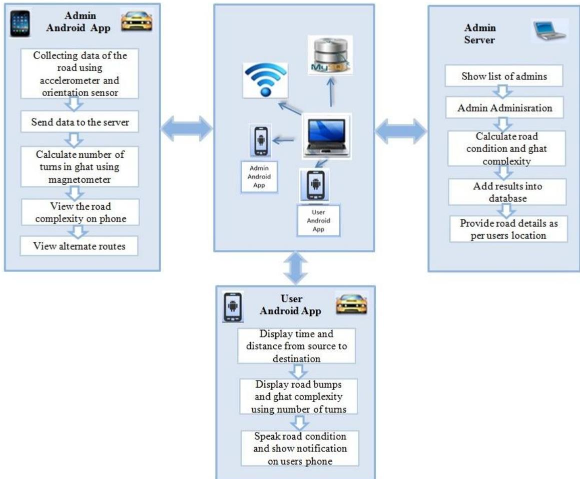
**Figure 3** System Architecture
