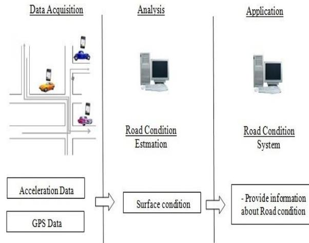
**Figure 1** Conceptual image of road condition system
