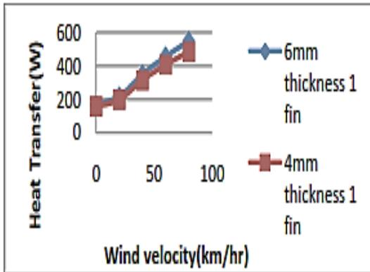
**Fig.1.** Heat transfer vs. air velocity for 6mm and 4mm thickness 1 no. of fin. [2]
