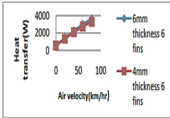
**Fig.4.** Heat transfer vs. air velocity for 6mm and 4mm thickness 6 no. of fin. [2].
