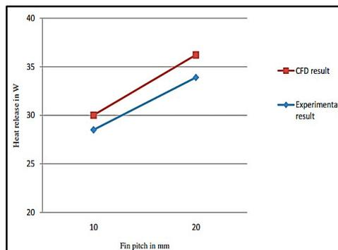
**Fig.5.** Comparison between experimental and CFD results [3]
