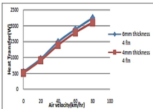
**Fig.3.** Heat transfer vs. air velocity for 6mm and 4mm thickness 4 no. of fin. [2].
