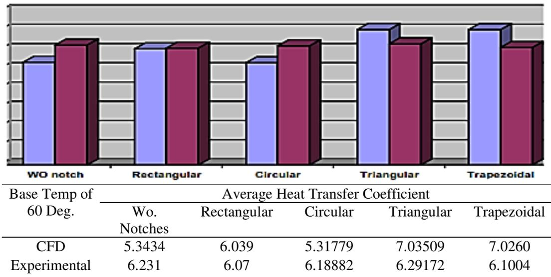
**Fig.6.** Comparison of heat transfer coefficient (HTC) by CFD and HTC by experiment [7]
