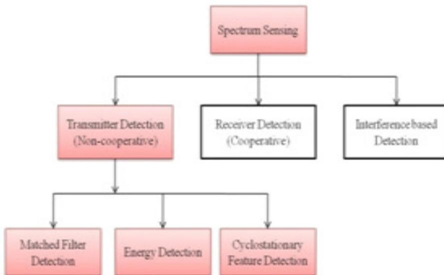
**Fig.2 Classification of Spectrum Sensing Techniques**
