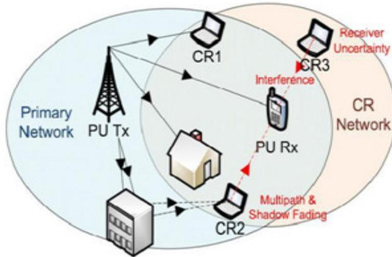
**Fig 6. Receiver Uncertainty and Multipath/Shadow Fading**
