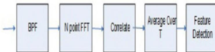
**Fig 5. Cyclostationary feature detector block diagram**
