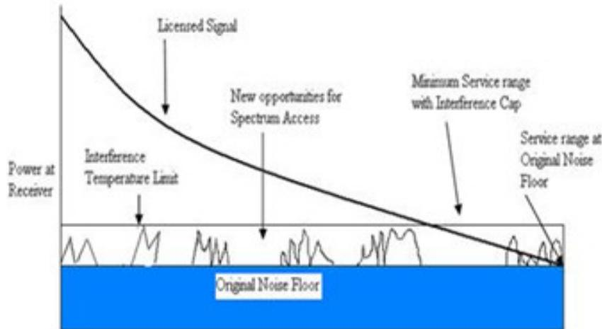
**Fig7. Interference temperature model**
