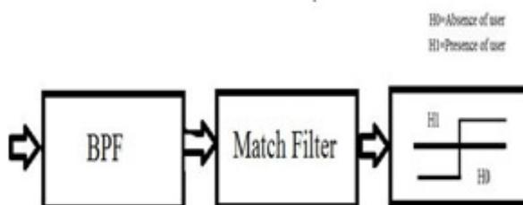
**Fig 3. Block diagram of matched filter**
