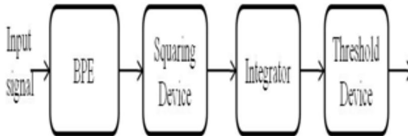
Fig 4. Energy detector block diagram
