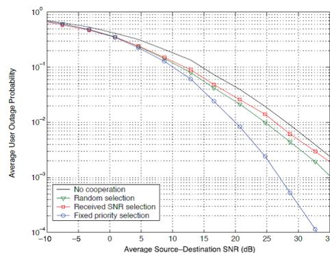
Figure: 3 Comparison of outage probability comparison of distributed & centralized techniques
