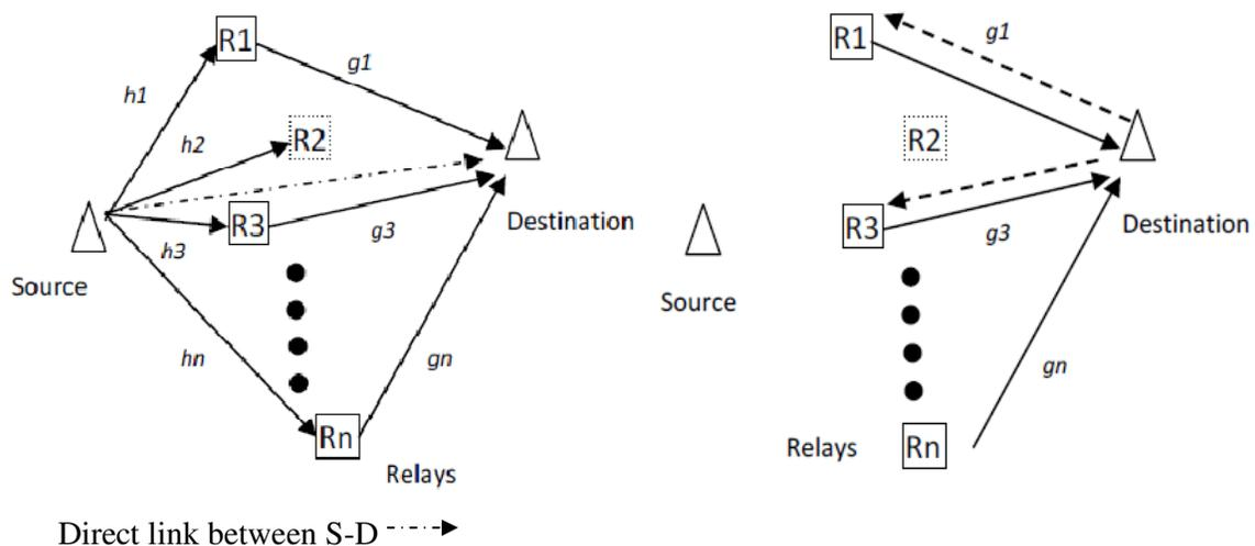
Fig. 1 General procedure of Cooperative Transmission relay selection
