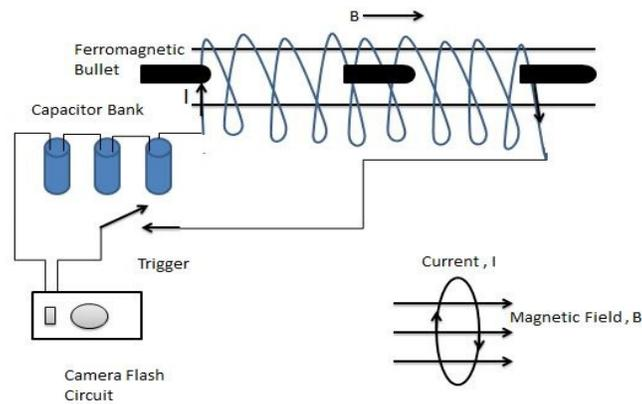
**Fig.4: Working principle of shooting mechanism**
