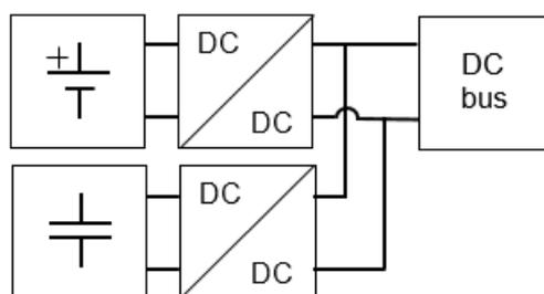
**Figure 1** Active parallel flowchart of hybrid energy storage
