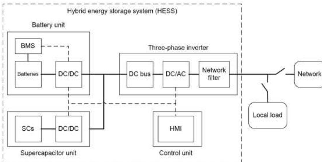
**Figure 2** Hybrid energy storage scheme: BMS – battery management system, SCs – supercapacitors, HMI – human-machine interface, DC/DC – dc-to-dc power converter, DC/AC – three-phase power inverter (dc-to-ac power converter).
