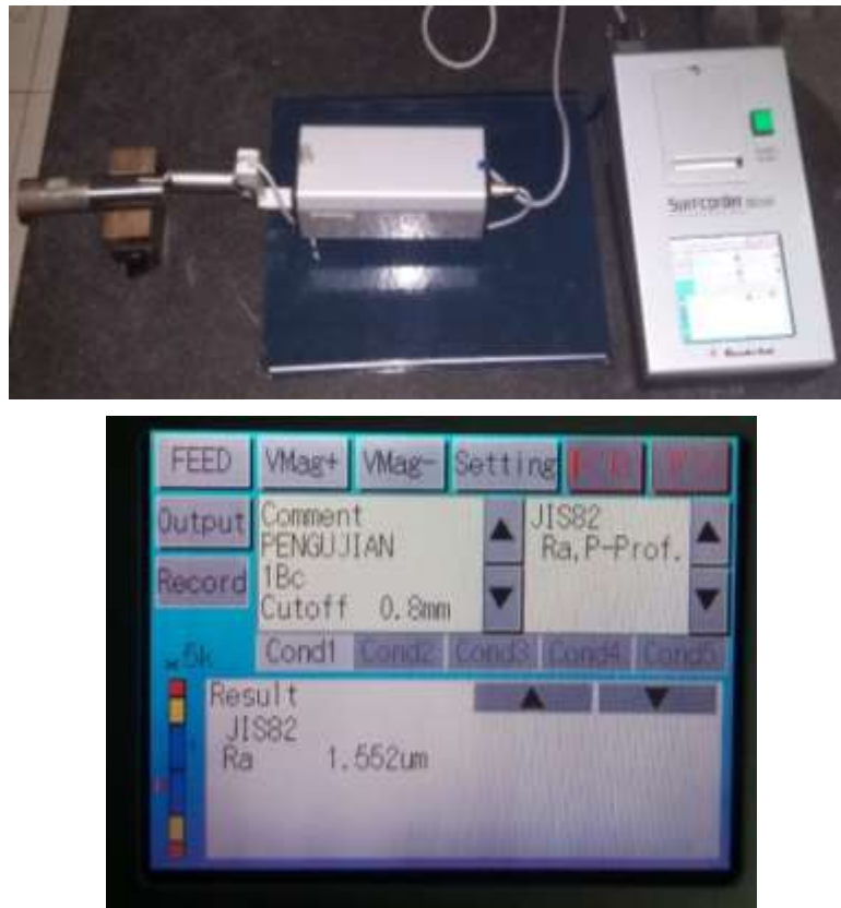
Figure 4 The process of surface roughness testing
