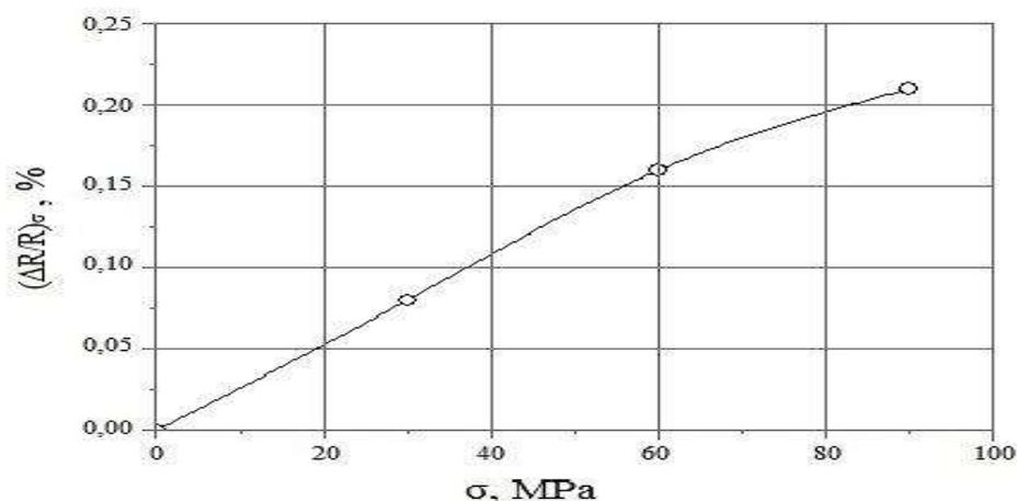
**Figure 13.** Dependence of the value  $\left(\frac{\Delta R}{R}\right)_\sigma$  on the value of mechanical stresses for the Ta-Co<sub>50</sub>Fe<sub>50</sub>-Ta nanostructure after annealing at 350°C
