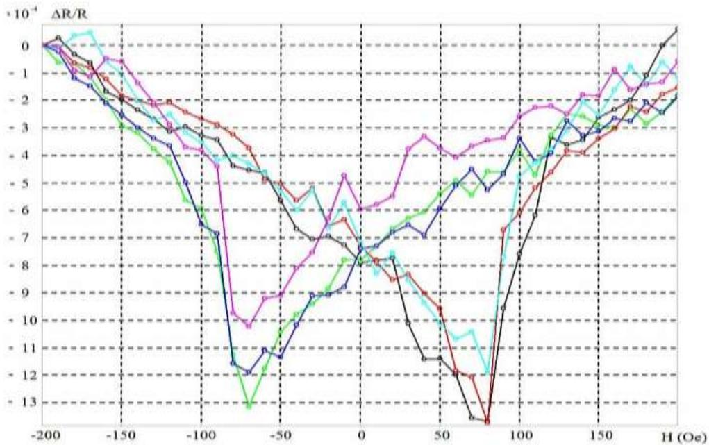
**Figure 10.** Measurement of the AMP effect under mechanical load of a  $\text{Co}_{50}\text{Fe}_{50}$  sample annealed at  $250^\circ\text{C}$ : blue, crimson – no load; red, blue, –  $\sigma = 30$  MPa; black, green –  $\sigma = 60$  MPa
