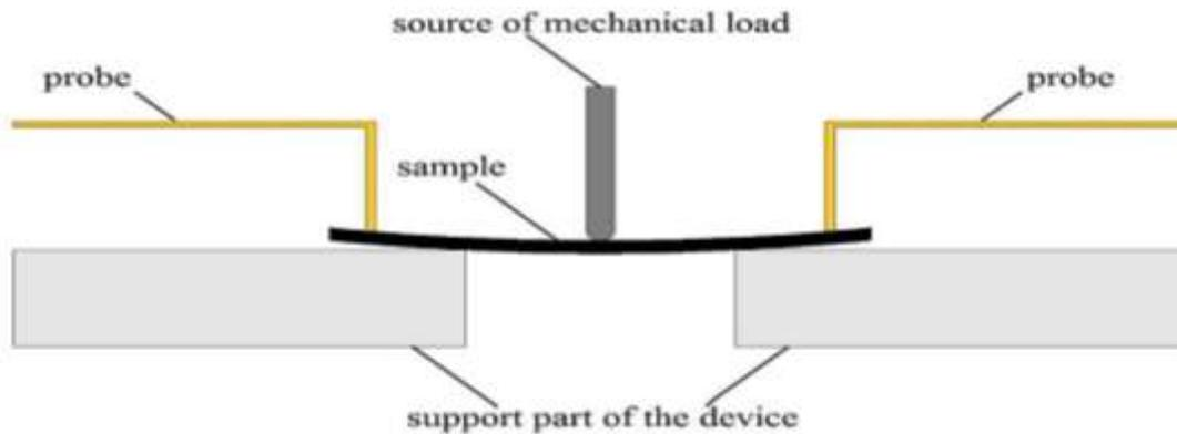
**Figure 1** Schematic representation of the main setup unit of the AMR measurement
