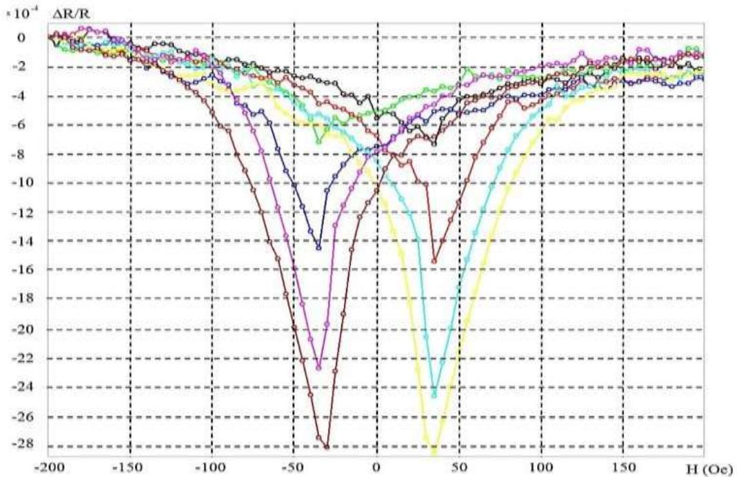
**Figure 11.** Measurement of the AMP effect under mechanical load of a  $\text{Co}_{50}\text{Fe}_{50}$  sample annealed at  $350^\circ\text{C}$ : black, green – no load; red, blue, –  $\sigma = 30$  MPa; blue, crimson –  $\sigma = 60$  MPa; yellow, brown –  $\sigma = 90$  MPa
