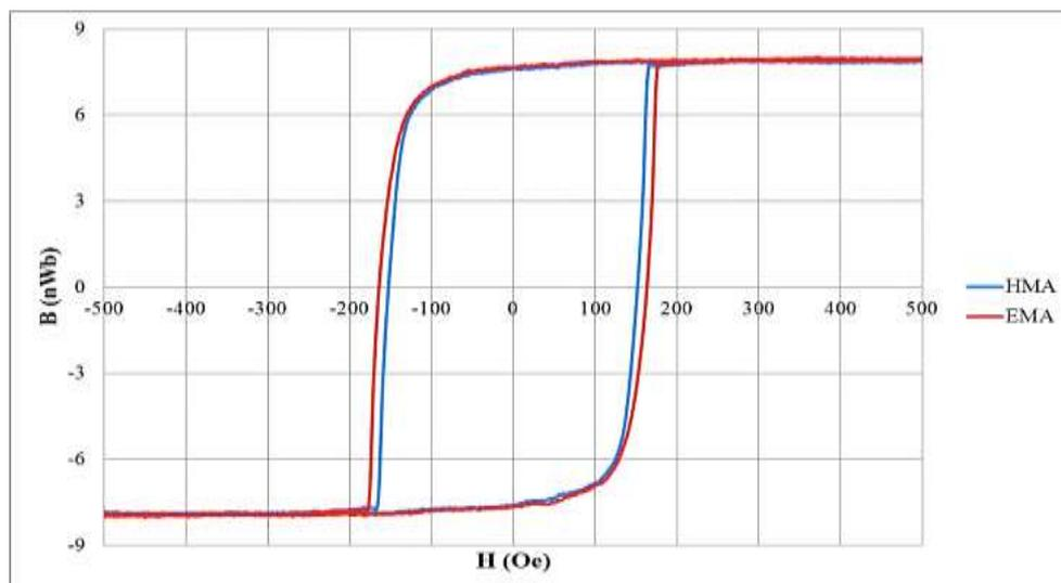
**Figure 6.** Dependence B(H) for the Co<sub>66</sub>Fe<sub>34</sub> layer before annealing
