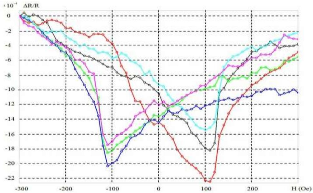
**Figure 9.** Measurement of the AMP effect under mechanical loading of the original  $\text{Co}_{50}\text{Fe}_{50}$  sample: blue, crimson – no load; black, green –  $\sigma = 30$  MPa; red, blue –  $\sigma = 60$  MPa
