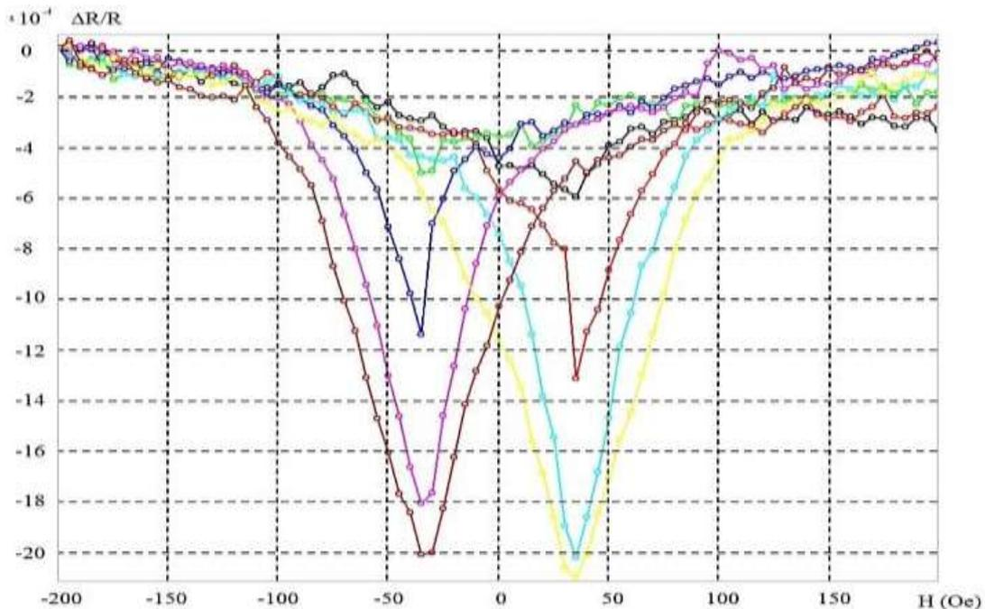
**Figure 12.** Measurement of the AMP effect under mechanical load of a  $\text{Co}_{50}\text{Fe}_{50}$  sample annealed at  $400^\circ\text{C}$ : black, green – no load; red, blue, –  $\sigma = 30$  MPa; blue, crimson –  $\sigma = 60$  MPa; yellow, brown –  $\sigma = 90$  MPa
