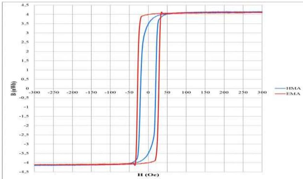
**Figure 3.** Dependence B (H) for the  $\text{Co}_{95}\text{Fe}_5$  layer before annealing
