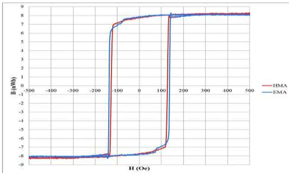
**Figure 8.** Dependence  $B(H)$  for the  $\text{Co}_{50}\text{Fe}_{50}$  layer before annealing
