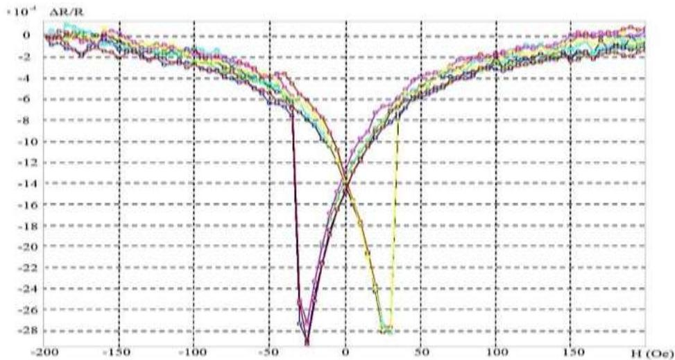
**Figure 5.** Dependence of the relative change in resistance of the initial Ta-Co<sub>95</sub>Fe<sub>5</sub>-Ta nanostructure on the value after annealing at temperature of 350°C: black, green – no load; red, blue –  $\sigma = 30$  MPa; blue, crimson –  $\sigma = 60$  MPa; yellow, brown –  $\sigma = 90$  MPa
