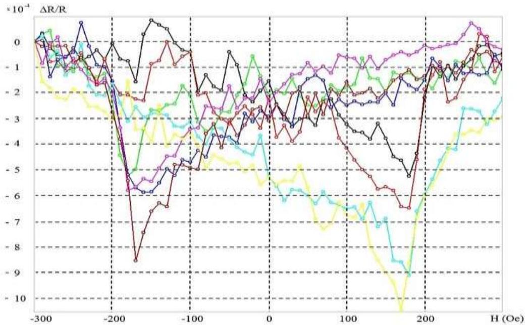
**Figure 7.** Measurement of the AMP effect under mechanical load of a sample annealed at 400°C of a  $\text{Co}_{66}\text{Fe}_{34}$  sample: black, green – no load; red, blue –  $\sigma = 30$  MPa; blue, crimson –  $\sigma = 60$  MPa; yellow, brown –  $\sigma = 90$  MPa
