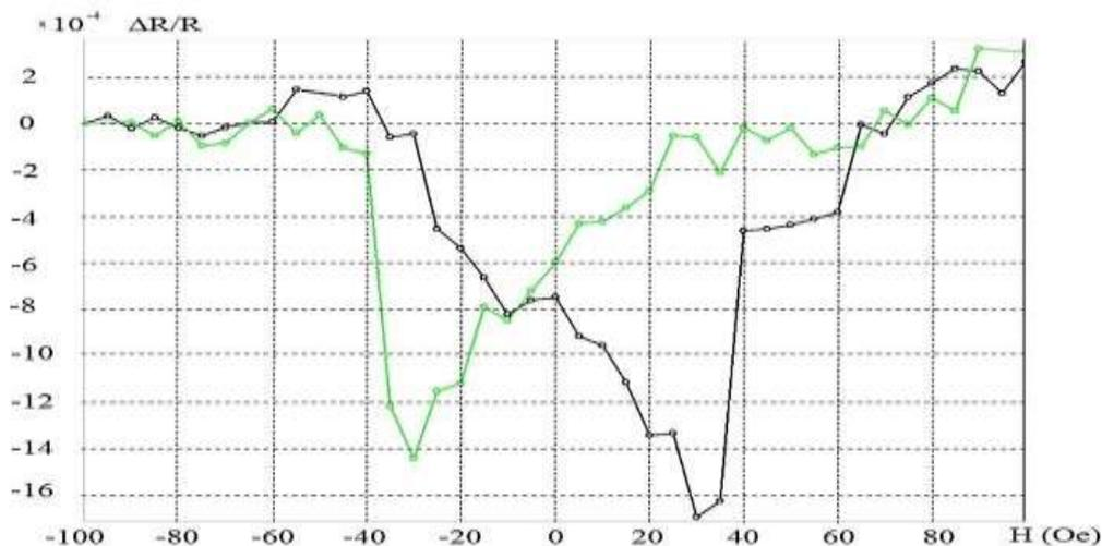
**Figure 4** Dependence of the relative change in resistance of the initial Ta- $\text{Co}_{95}\text{Fe}_5$ -Ta nanostructure on the value of external magnetic field: black – straight motion; green – reverse one
