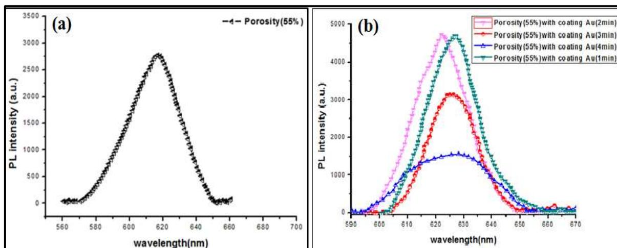
**Figure 5** Shows the PL spectra of a) as formed mesoPSi b) AuNPs/PS deposited at  $C= 5 \times 10^{-3}$  M diluted in HF
