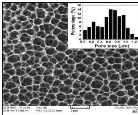
**Figure 3** SEM images showing (top view) of as formed mesoPSi with the statistical distribution of pores prepared nanoporous surface prepared at etching time 20 min.
