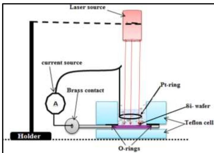
**Figure 1** The Experimental setup of a photo-electrochemical etching technique.
