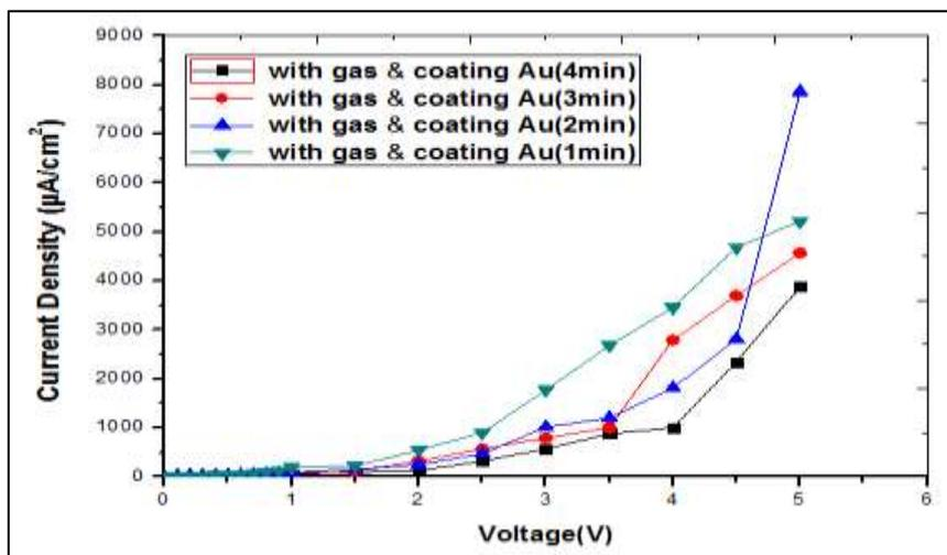
Figure 8 I-V Characteristics of Al/AuNPs/mesoPSi/Al structure with different coating gold nanoparticles after NH<sub>3</sub> exposure at room temperature.
