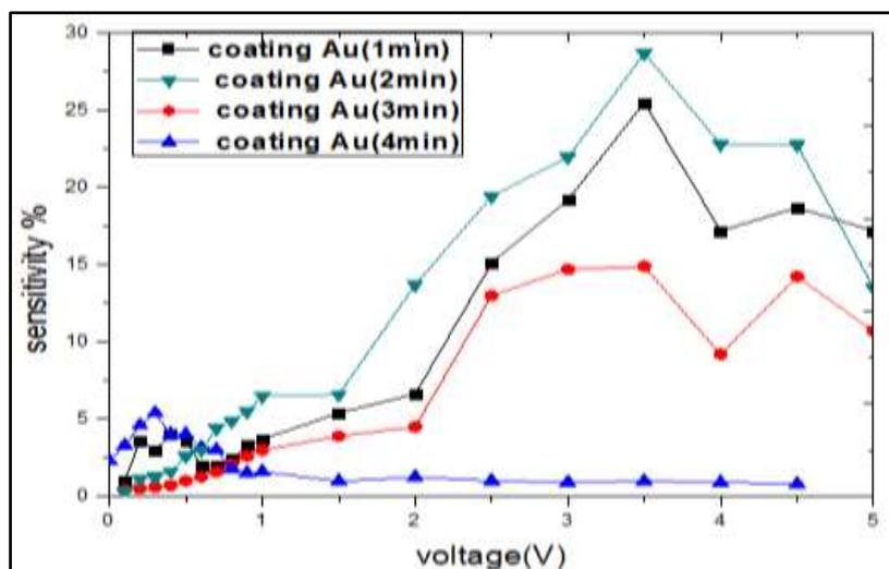
**Figure 10** Sensitivity-voltage characteristics of Al/AuNPs/Psi /Al structure with different coating gold nanoparticles after NH<sub>3</sub> exposure at room temperature.
