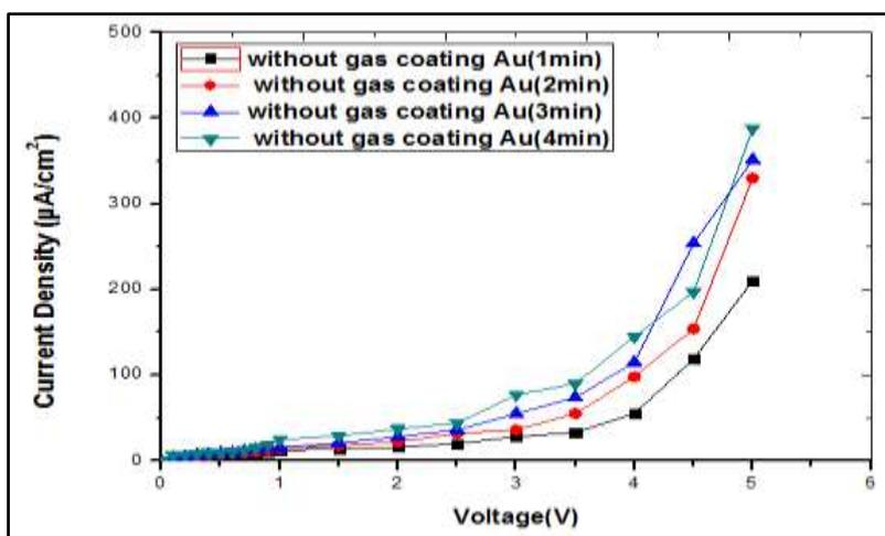
Figure 7 I-V Characteristics structure with different coating gold nanoparticles before NH<sub>3</sub> exposure at room temperature.
