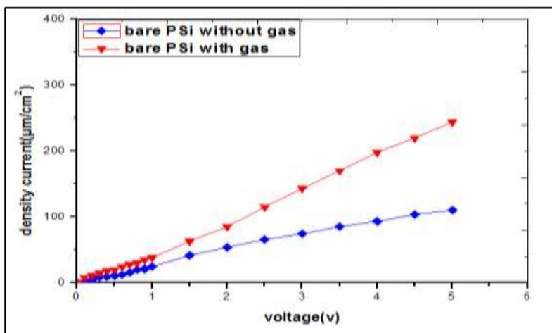
Figure 6 I-V characteristics structure for bare PSi at without gas and with gas at room temperature.
