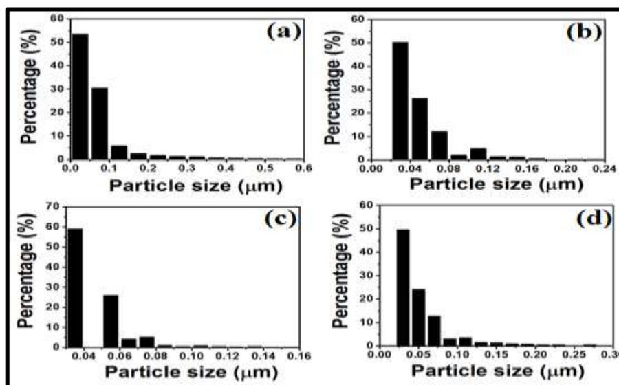
**Figure 4** SEM images of gold layer deposited on porous silicon from  $\text{HAuCl}_4$  (1m M)/3Mm HF the solution at different dipping times a)1 min (b)2 min (c) 3 min (d)4 min with the statistical distribution of particle size.
