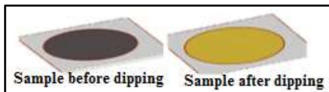
**Figure 2** Shows the images of Psi samples before and after dipping prepared by a photo-electrochemical etching technique.
