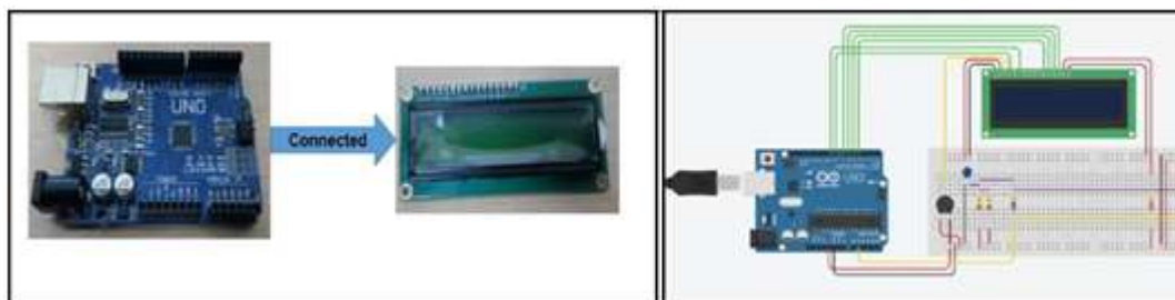
Figure 3 Circuit diagram of LCD display connected to main board.
