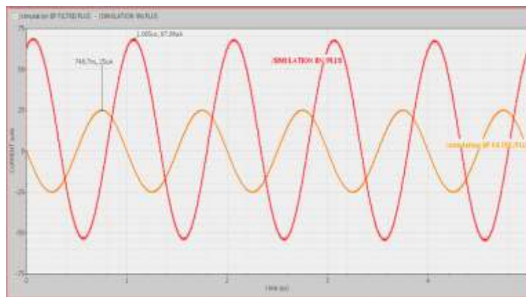
Figure 10 Time domain response of current-mode bandpass filter output
