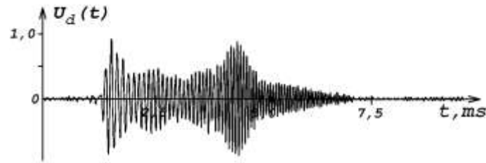
Figure 8 a Chirp signal U_d(t) distorted in electroacoustic path
