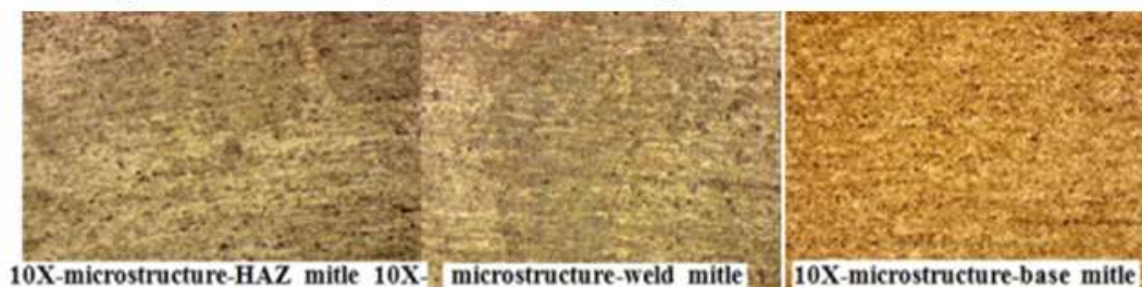
Fif.5. the microstrucure the specimens welding in FWS of welding method.
