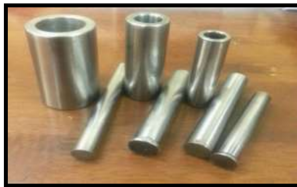
Figure 2 Die, Punch, and a Holder for Mold.
