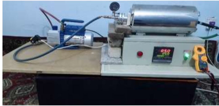
Figure 6 Electrical Furnace with a Vacuum System
