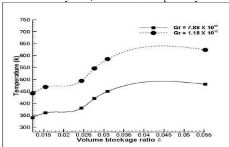
**Figure 8** Variation of average temperature with volume blockage ratio  $\delta$
