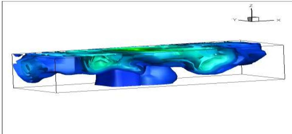
**Figure 4** Iso-surface of thermal plumes
