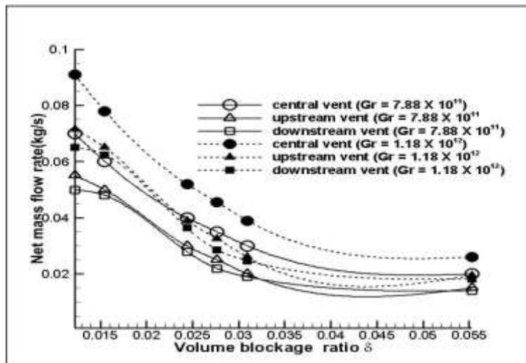
Figure 7 Variation of net mass flow rate with volume blockage ratio ( $\delta$ )
