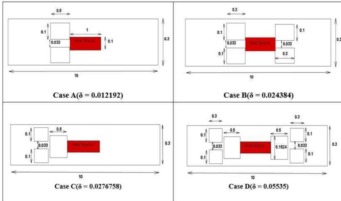
**Figure 2** Top view of the channel with various arrangements of obstacles (all dimensions are in m)
