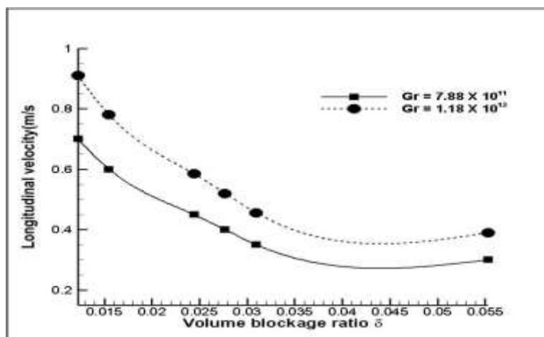
**Figure 9** Variation of average longitudinal velocity with volume blockage ratio ( $\delta$ )
