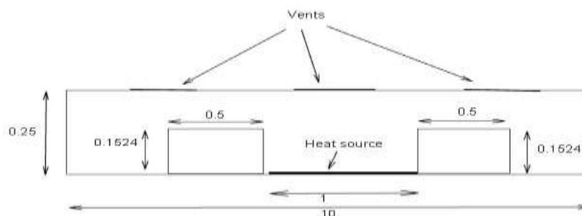
**Figure 1** Schematic diagram of channel: Front view (all dimensions are in m)
