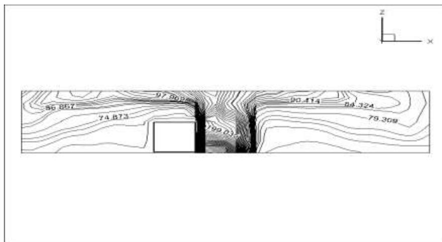
**Figure 5** Variation of temperature contours along the length of tunnel in  $^{\circ}\text{C}$
