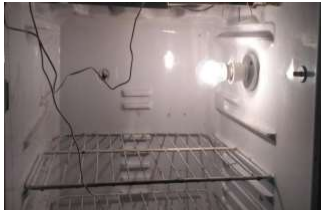
Figure 3 Loading Condition with 100Watt bulb
