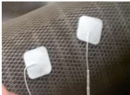
Figure 5.6 Electrode mounting on air filter
