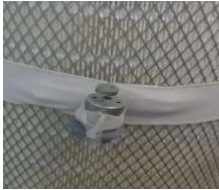
Figure 5.10 Vibration motor mounted using elastic harness
