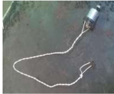
Figure 5.9 Vibration motor after extension
