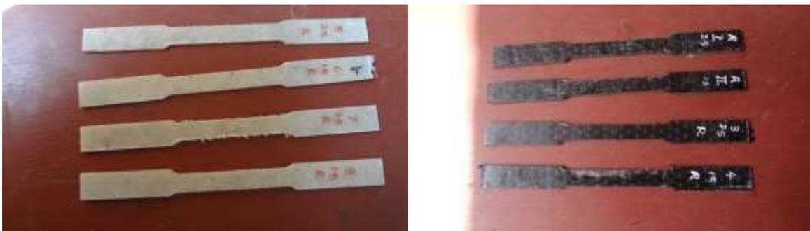
**Figure 6** Tensile Samples of glass and Carbon Fiber Before testing
