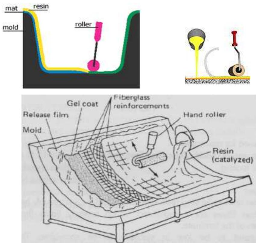
**Figure 1** Hand lay-up Method
