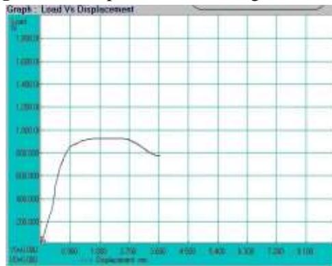
Figure 14 Sample-4 Strain Rating 1.5mm/min
