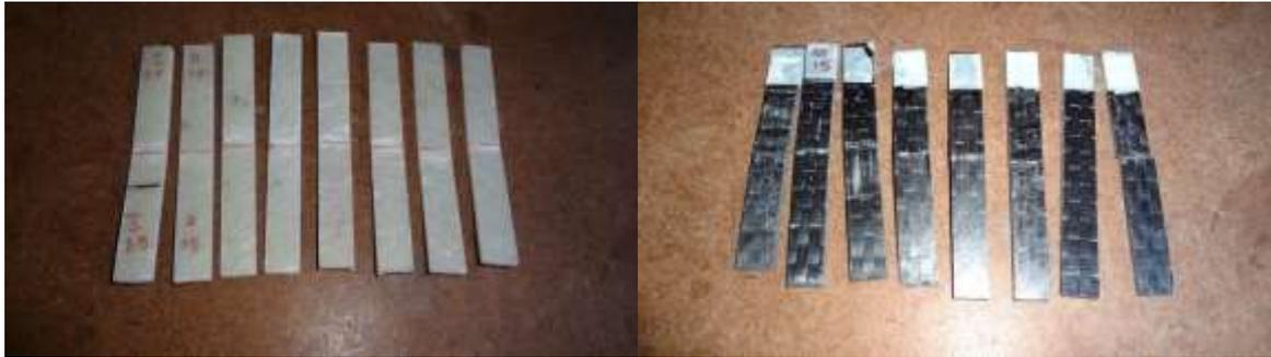
**Figure 9** Flexural specimen for glass and carbon fiber after testing
