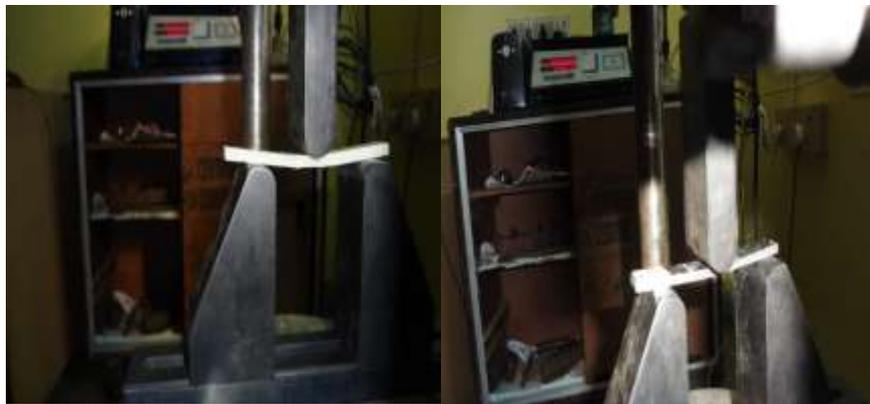
**Figure 10** Flexural test for glass and carbon fiber
