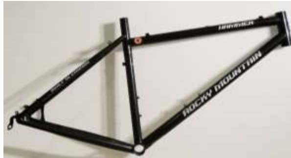
Figure 1 Frame construction of mountain bike in the form of diamond
