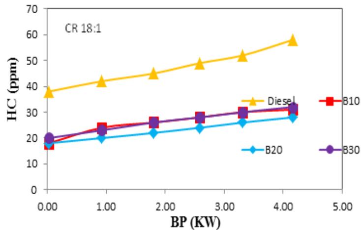
Figure 6 Brake power Vs HC
