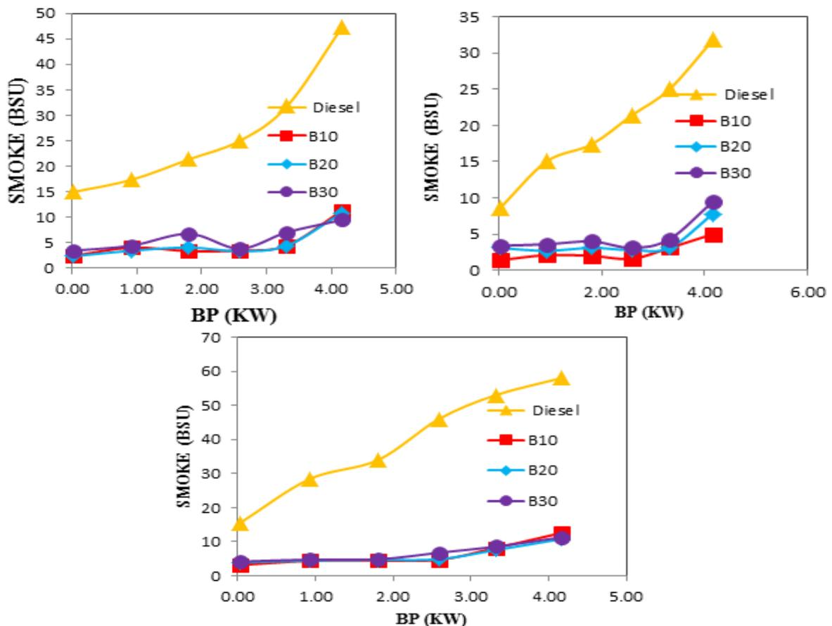
Figure 7 Brake power Vs Smoke
