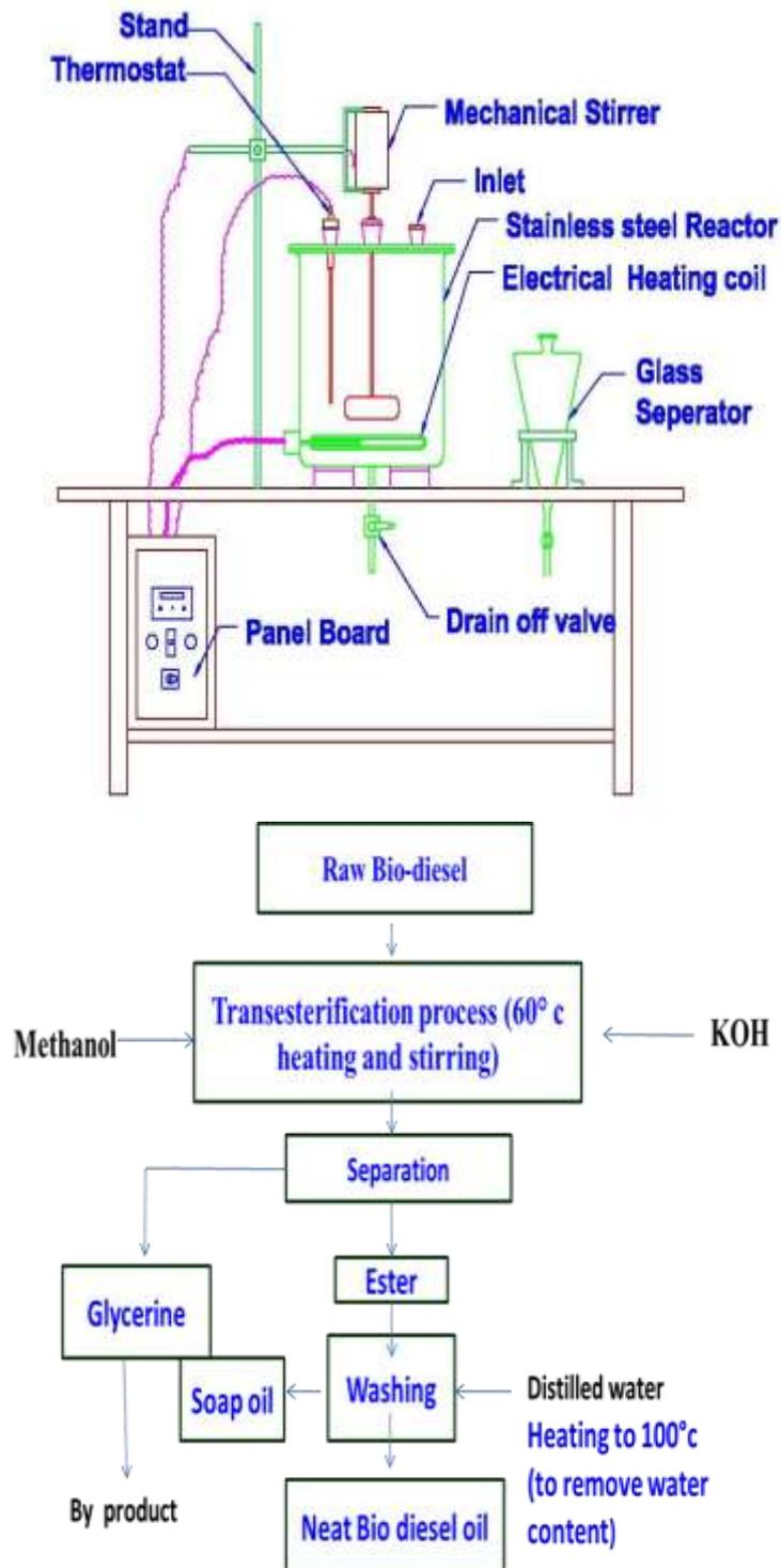
**Figure 2** Experimental setup for production of biodiesel and Flow Chart of Bio-Diesel Trans-esterification Process
