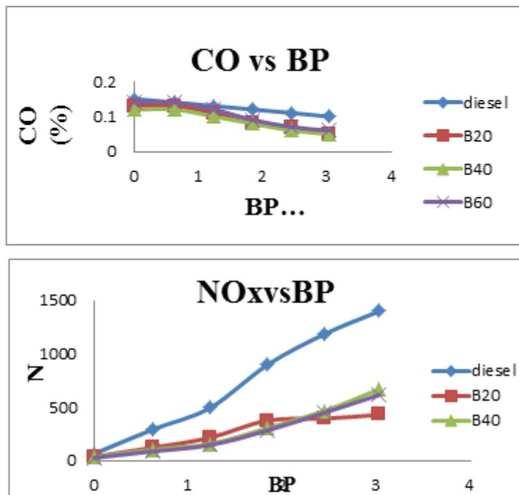
From the Fig shows that the variations of element oxides (NOx) emission with load for various blends. The Night emission for biodiesel and its blends is not up to that of ordinary diesel at numerous BP. the rationale for lesser Night emission for blends is attributable to the lower peak temperature.
