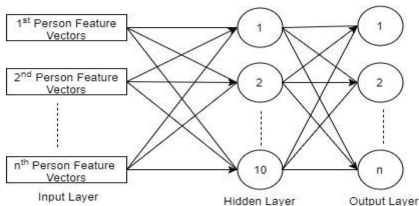
Figure 2 Structural design of Neural Networks
