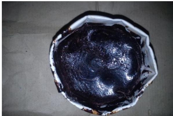
**Figure 4** CNSL resin for composite
