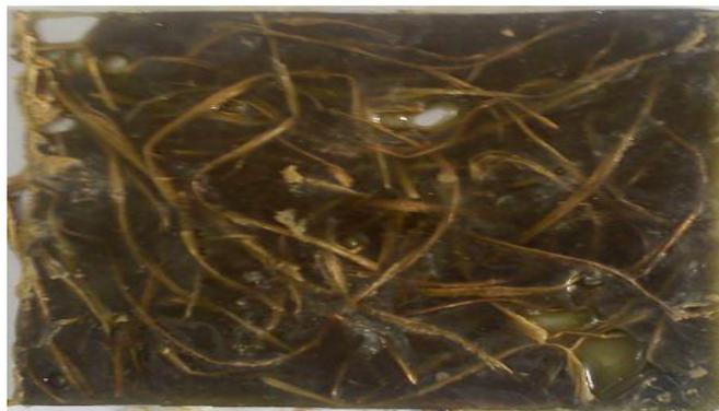
**Figure 1** Composite with banana fiber and synthetic resin
