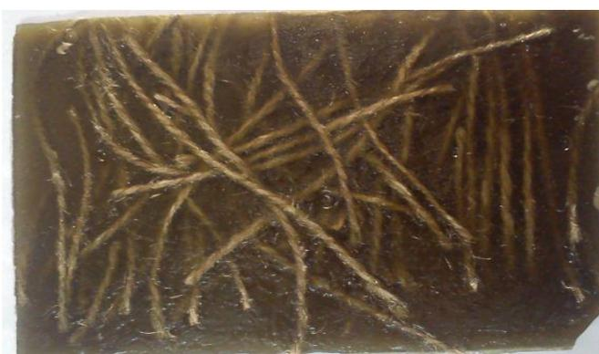
**Figure 2** Composite with jute fiber and synthetic resin
