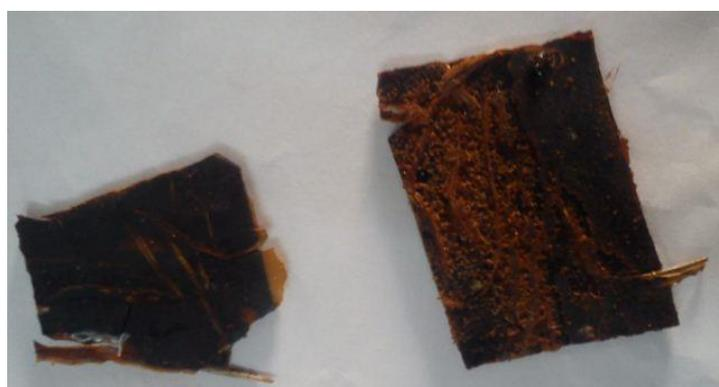
**Figure 3** Composite with jute, banana fiber and blended resin
