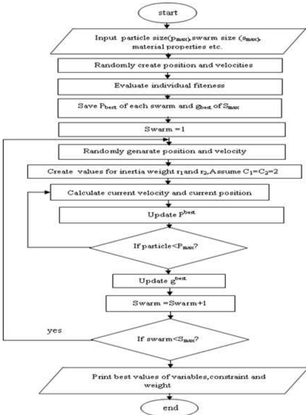
**Figure 5** Flowchart of PSA based Optimal Design of Skid landing Gear.
