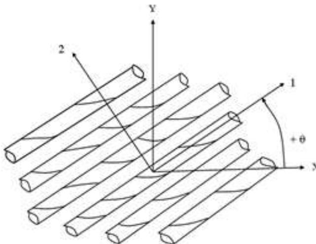
**Figure 2** lamina with arbitrary orientation
