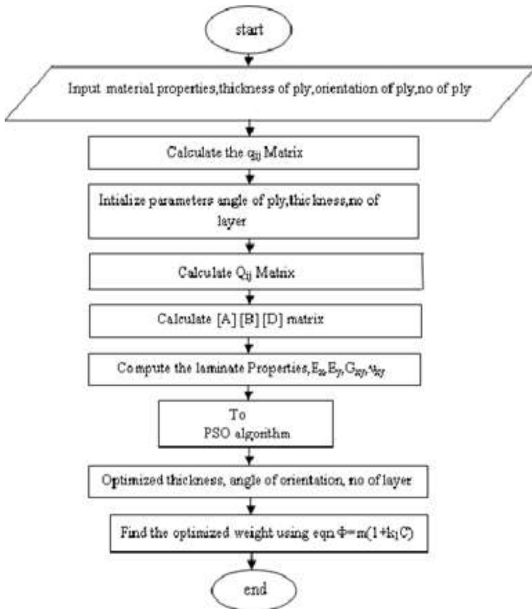
**Figure 4** Design algorithm of skid Landing Gear
