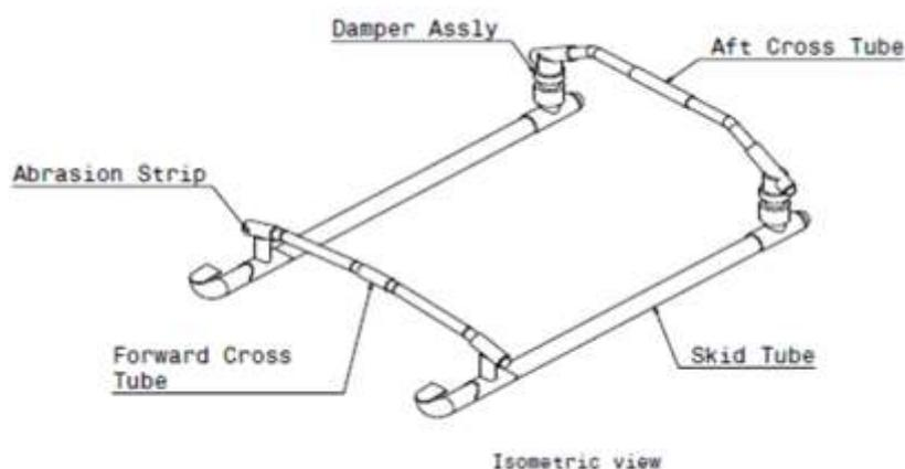
Figure 1 Skid landing Gear
