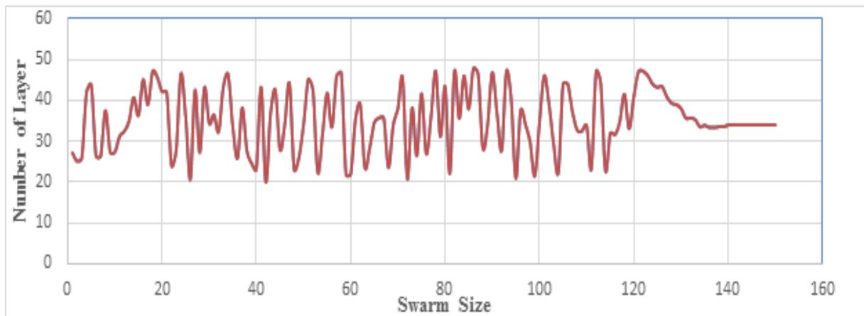
**Figure 7** Variations of number of layers of Kelvar49 Epoxy skid Tubes with Swarm Size
