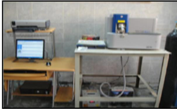
**Figure 1:** Material analyzer (spectrometer) type spectromax
