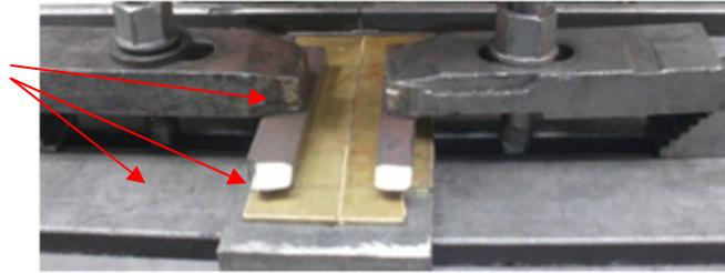
**Figure 3:** The designed clamping device
