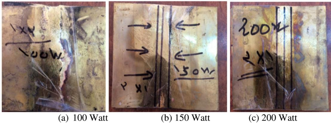
**Figure 5:** Laser welding Joint of Brass for different power
