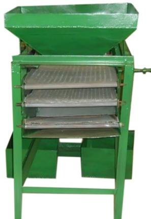
**Plate 2:** Front view of the cleaner grader showing deflector in between the middle and bottom sieves
