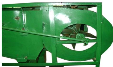
**Plate 3:** Blower assembly at 5° inclination to the horizontal
