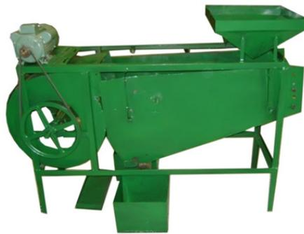
**Plate 1:** Side view of the cleaner grader
