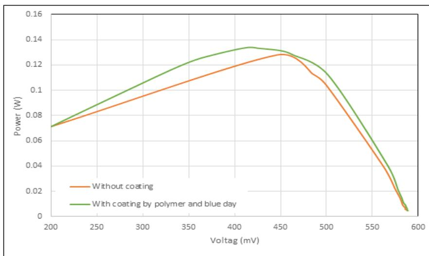
**Figure 8** The relationship between power and voltage with and without coating.
