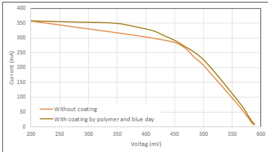
**Figure 6** The relationship between voltage and current with and without coating.
