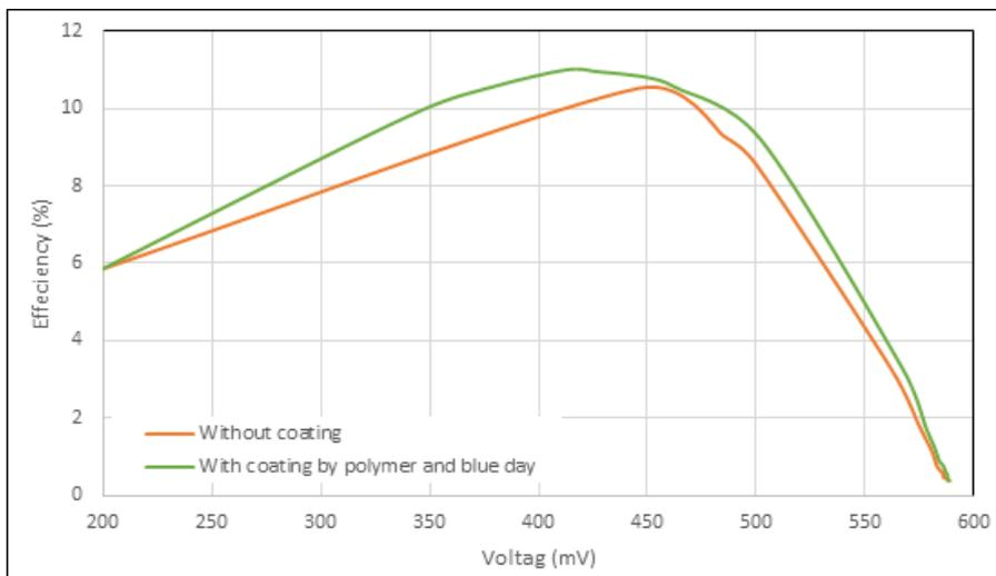
**Figure 7** The relationship between efficiency and voltage with and without coating.
