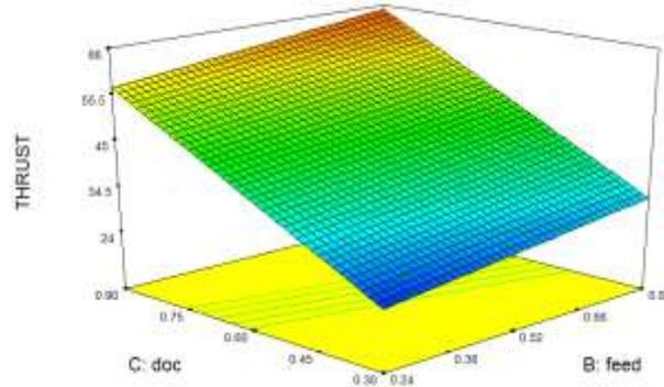
Figure 11 Depth of Cut Vs Feed Rate on Thrust Force.
