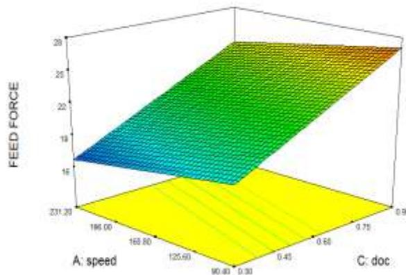
Figure 7 Spindle Speed Vs Depth of Cut on Feed Force
