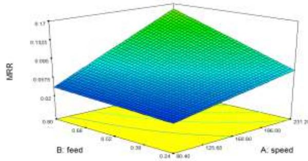
**Figure 3** Spindle speed Vs feed on MRR
