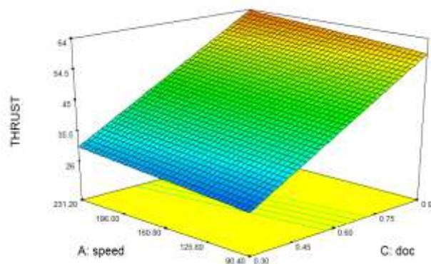
**Figure 10** Spindle Speed Vs Depth of Cut on Thrust Force
