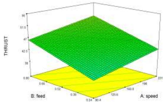
**Figure 9** Feed Rate Vs Spindle Speed on Thrust Force
