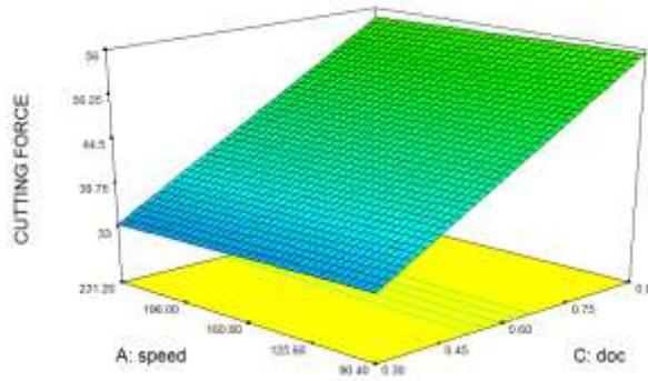
Figure 13 Spindle Speed Vs Depth of Cut on Cutting Force
