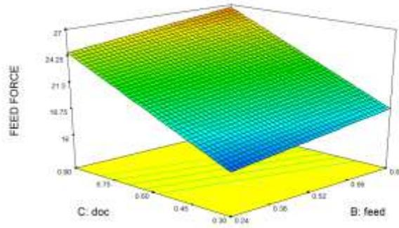
**Figure 8** Depth of cut Vs Feed Rate on Feed Force
