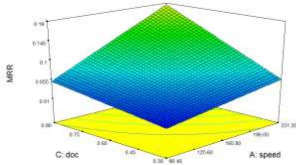
**Figure 4** Spindle speed Vs Depth of cut on MRR
