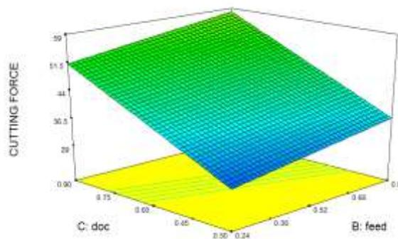
Figure 14 Depth of cut Vs Feed Rate on Cutting Force
