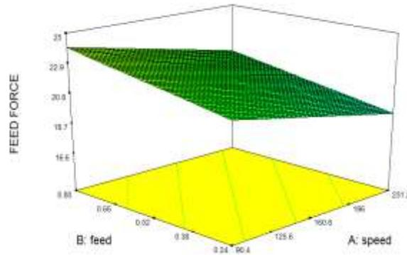
Figure 6 Spindle speed Vs Feed rate on Feed Force
