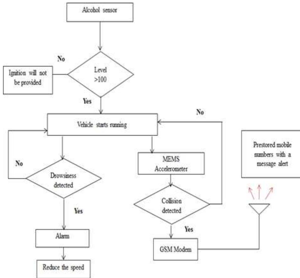
**Figure 3.** Flow diagram of the proposed model
