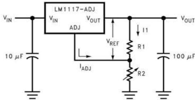
**Figure 2.** Circuit diagram of voltage regulator
