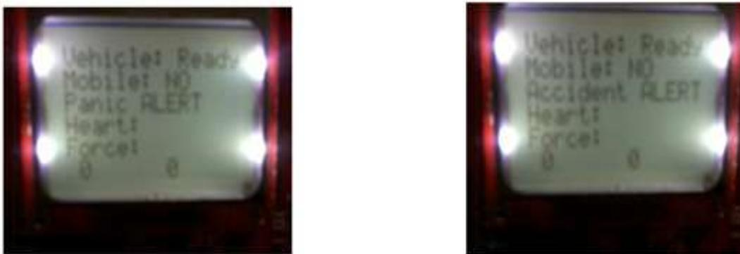
**Figure.8** Panic and accident alert outputs
