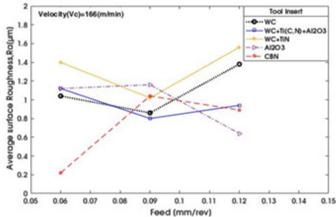
Fig.17 Surface Roughness vs. Feed at constant Speed (166 m/min), Feed (0.06, 0.09, 0.12 mm/rev)
