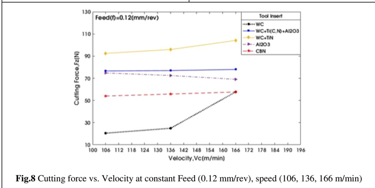
**Fig.8** Cutting force vs. Velocity at constant Feed (0.12 mm/rev), speed (106, 136, 166 m/min)
