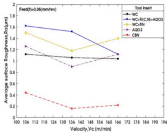
**Fig.12** Surface Roughness vs. Velocity at constant Feed (0.06 mm/rev), speed (106, 136, 166 m/min)
