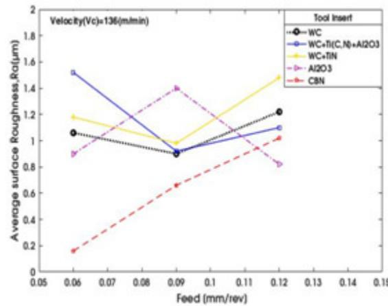
Fig.16 Surface Roughness vs. Feed at constant Speed (136 m/min), Feed (0.06, 0.09, 0.12 mm/rev)
