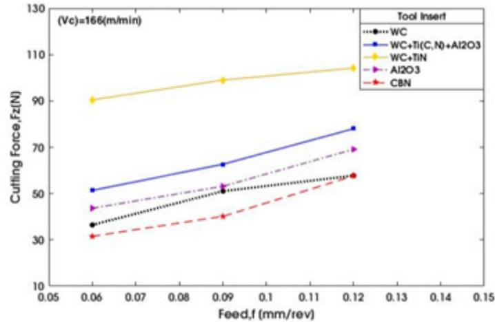
**Fig.11** Cutting force vs. Feed at constant Speed (166 m/min), Feed (0.06, 0.09, 0.12 mm/rev)
