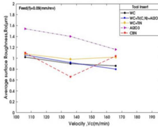
**Fig.13** Surface Roughness vs. Velocity at constant Feed (0.09 mm/rev), speed (106, 136, 166 m/min)
