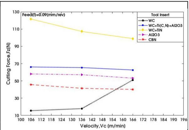
**Fig.7** Cutting force vs. Velocity at constant Feed (0.09 mm/rev), speed (106, 136, 166 m/min)
