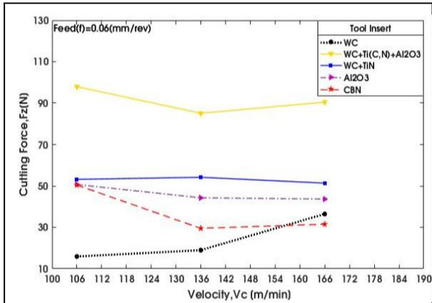
**Fig.6** Cutting force vs. Velocity at constant Feed (0.06 mm/rev), speed (106, 136, 166 m/min)
