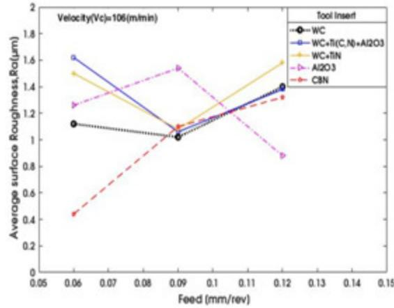
Fig.15 Surface Roughness vs. Feed at constant Speed (106 m/min), Feed (0.06, 0.09, 0.12 mm/rev)
