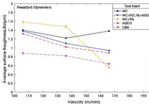
**Fig.14** Surface Roughness vs. Velocity at constant Feed (0.12 mm/rev), speed (106, 136, 166 m/min)
