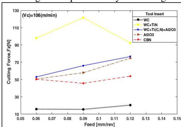
**Fig.9** Cutting force vs. Feed at constant Speed (106 m/min), Feed (0.06, 0.09, 0.12 mm/rev)
