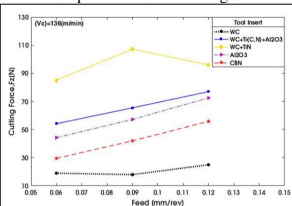
**Fig.10** Cutting force vs. Feed at constant Speed (136 m/min), Feed (0.06, 0.09, 0.12 mm/rev)
